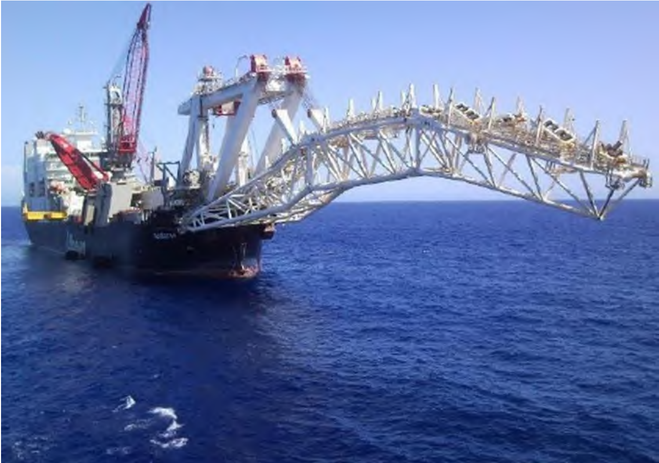
Figure 4-2: Conventional pipelay vessel
