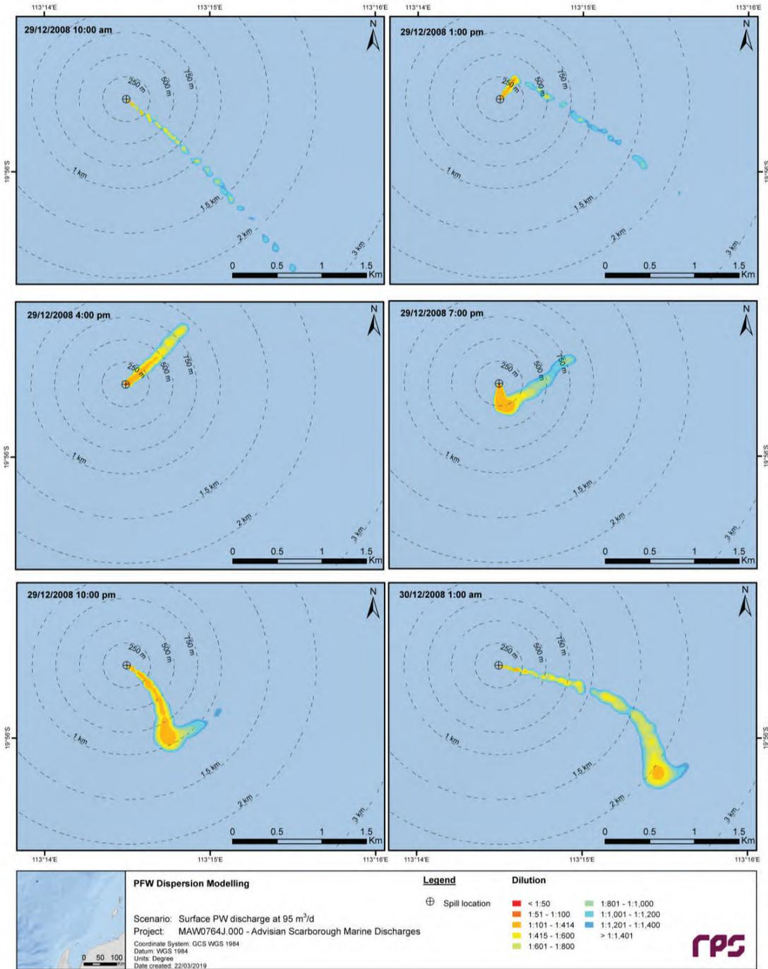
**Figure 3.13** Snapshots of predicted dilution levels, at 3-hour intervals from 10:00 on 29<sup>th</sup> December 2008 to 01:00 on 30<sup>th</sup> December 2008, for Case P1 (0 m depth discharge at 95 m<sup>3</sup>/d flow rate).
