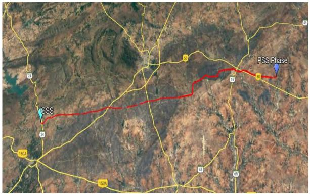
Figure 3-6: Transmission Line Route for the proposed project (PSS I to GSS)
