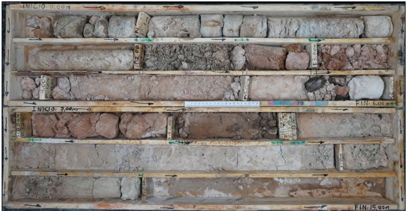
Figura C 7: Sondeo BH-08 0-15 m
