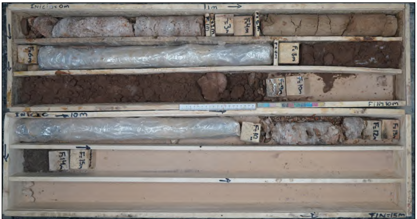
Figura C 5: Sondeo BH-06 0-15 m
