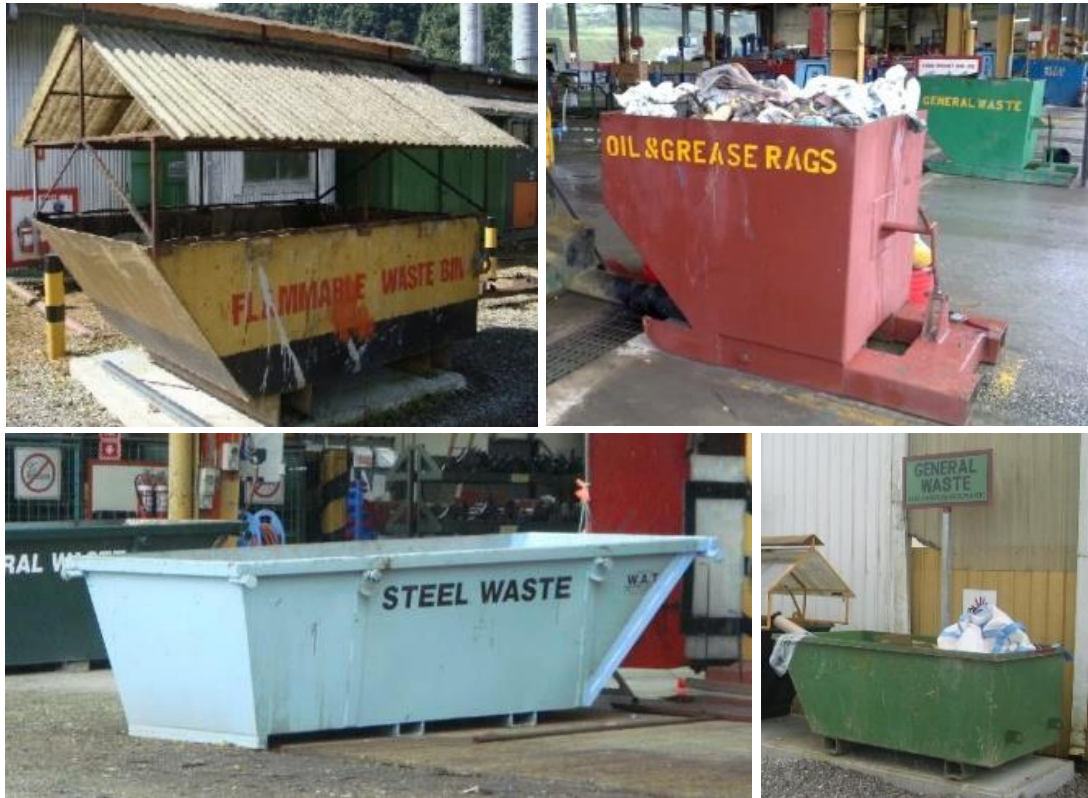
Figure 11 Examples of Correctly Coloured and Labelled Skips
