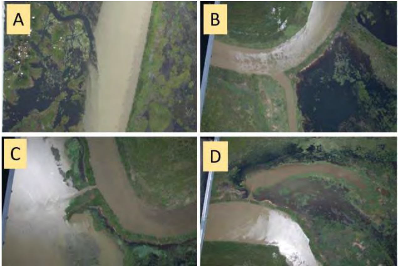
Figure 5-20. (A) Blocking of access of main river water by floodplain standing water. (B) Isolated floodplain ORWBs behind main channel and tie channel levees. (C) Inflow of main river water through a levee breach with levee backplain water immediately behind the levee unaffected. (D) Inflow of sediment laden water through a breach in a meander cutoff plug. Note how water in areas behind the cutoff channel levees is largely unaffected and remains relatively clear.
