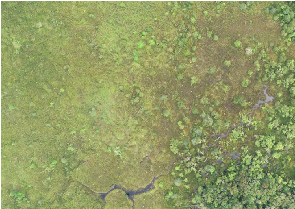
Fig.8-4: Swamp area with limited surface water yet showing SENTINEL DN values usually associated with 70-90% surface water. SENTINEL C-band radar appears to penetrate the plant cover. From Pickup and Marshall, (2019).
