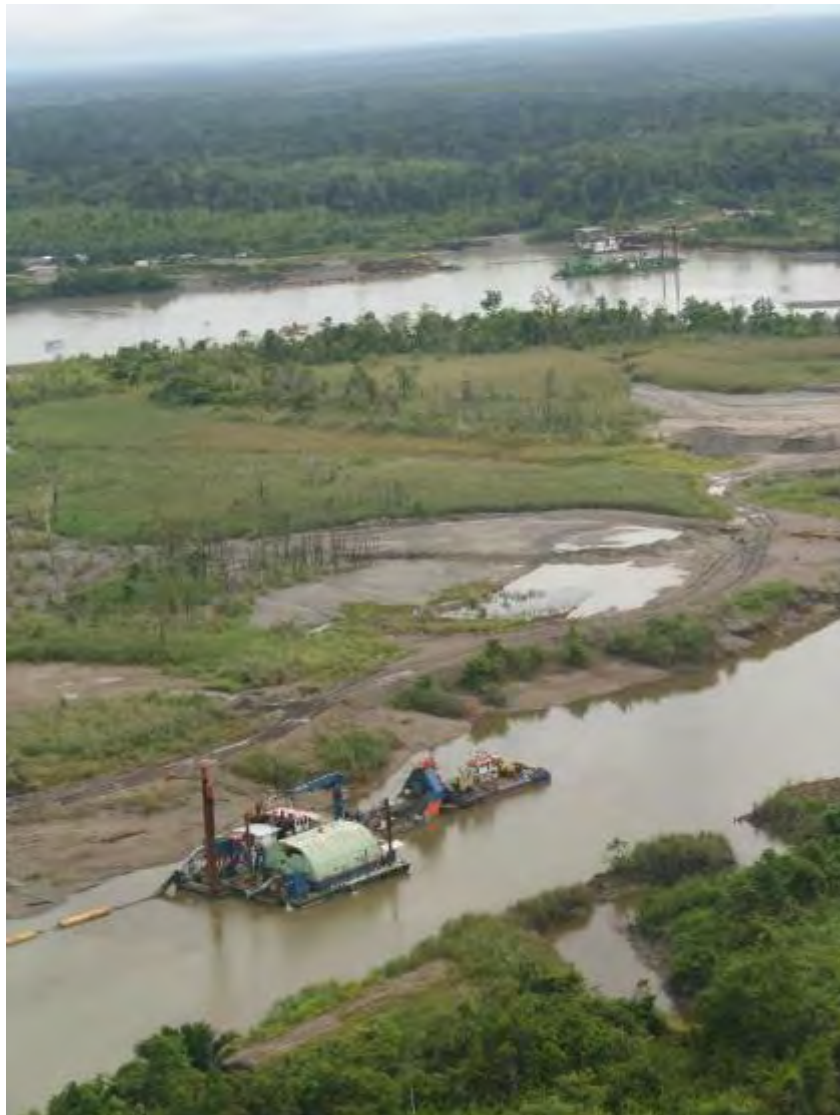
Figure 3-13. Dredging operations at Bige on the Lower Ok Tedi.
