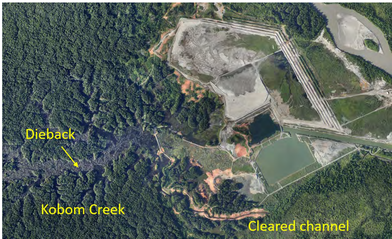
Figure 11.3. Kobom Creek and the Bige West Bank showing cleared areas, opened-up diversion channel and dieback area.
