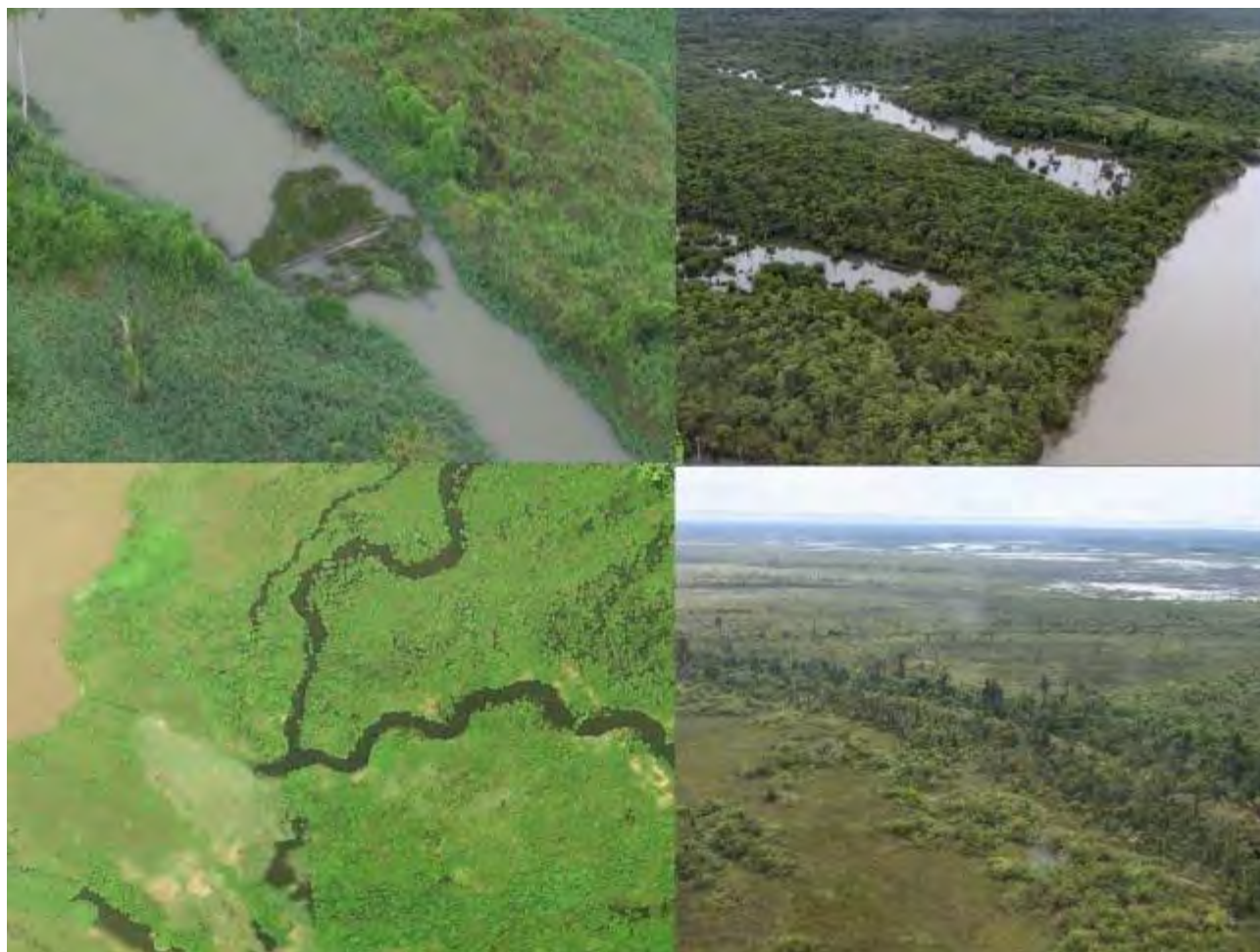
Figure 5-21. Examples of tie channel and ORWB blocking. Upper left: sediment accumulation and vegetation growth around a trapped log in a tie channel which may clear or may develop further. Upper right sediment plugs blocking access to a lake in a meander cutoff. Lower left: completely blocked tie channel next to the main river. Lower right: infilled former tie channel with tree growth on slightly raised former levees.
