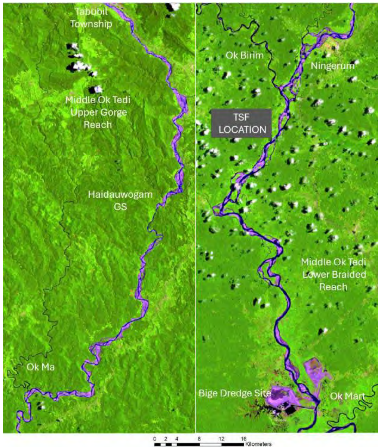
Figure 2-5. Landsat TM satellite image of the Middle Ok Tedi. The upper gorge section is on the left with the downstream braided section on the right. The transition to a single channel set in a floodplain occurs just after the Bige dredge site.
