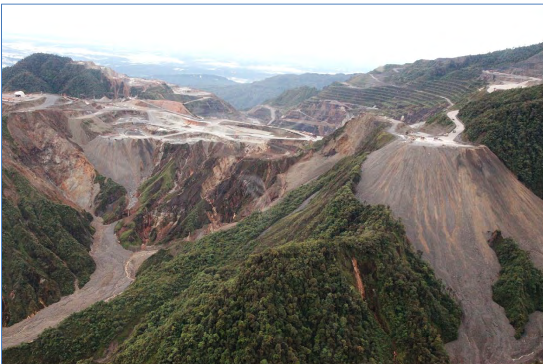
Figure 2: The new Northern Dump (left) showing a limited catchment area and limited toe losses. The Southern Dump (right) continues to have a high loss rate. Photos: January, 2014.
