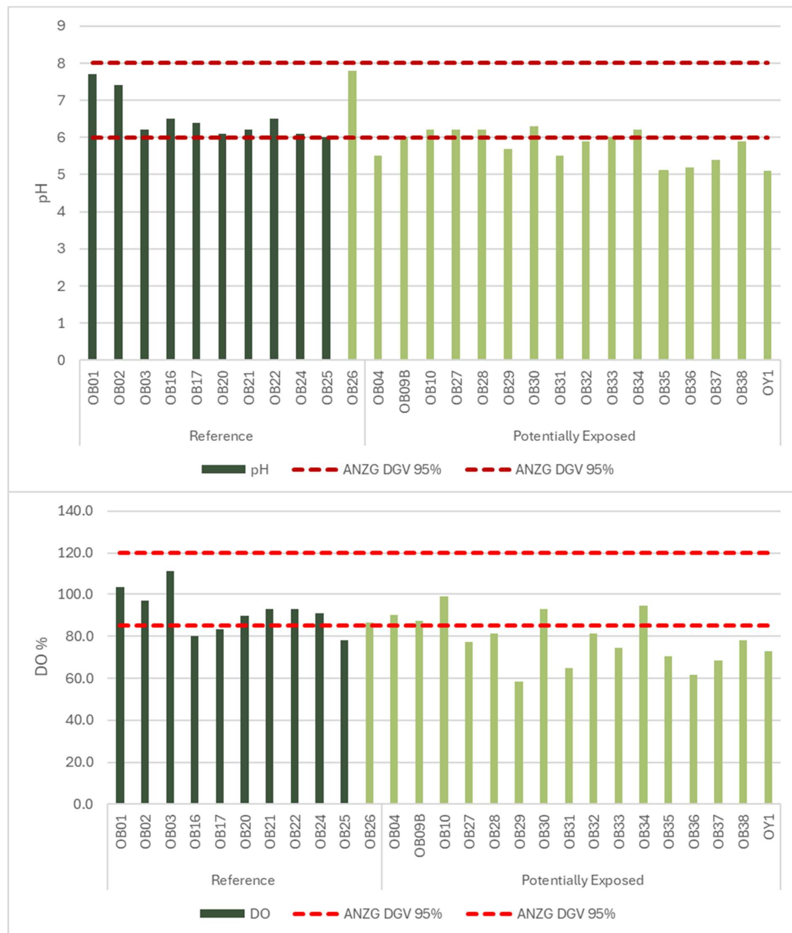
Figure 11. pH and Dissolved Oxygen Saturation (%) recorded from all sites sampled in comparison to the upper and lower ANZG 95% species protection default guideline values
