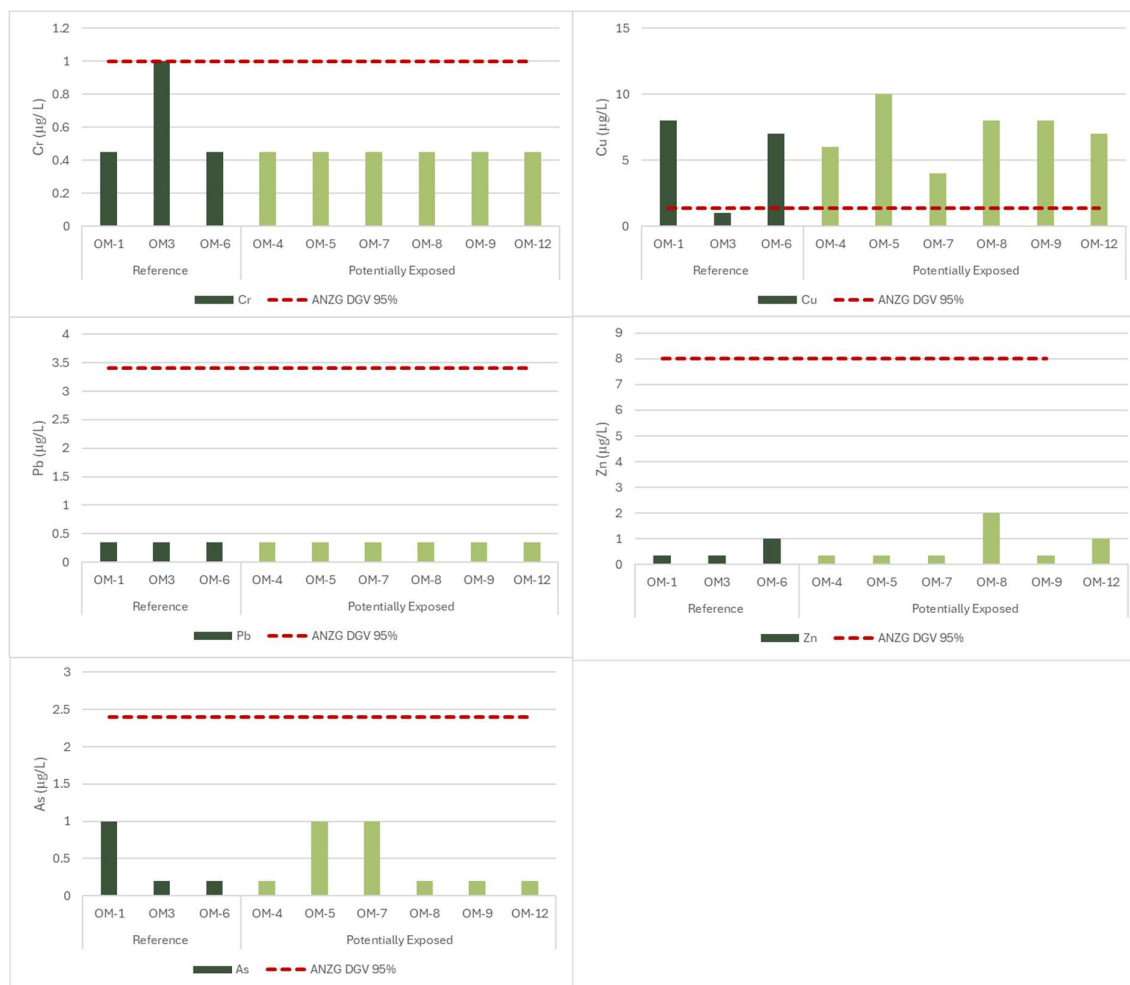
Figure 31. Dissolved metal concentrations (µg/L) in comparison to the 95% ANZG (2018) guidelines showing plots for dCr, dCu, dPb, dZn and dAs
