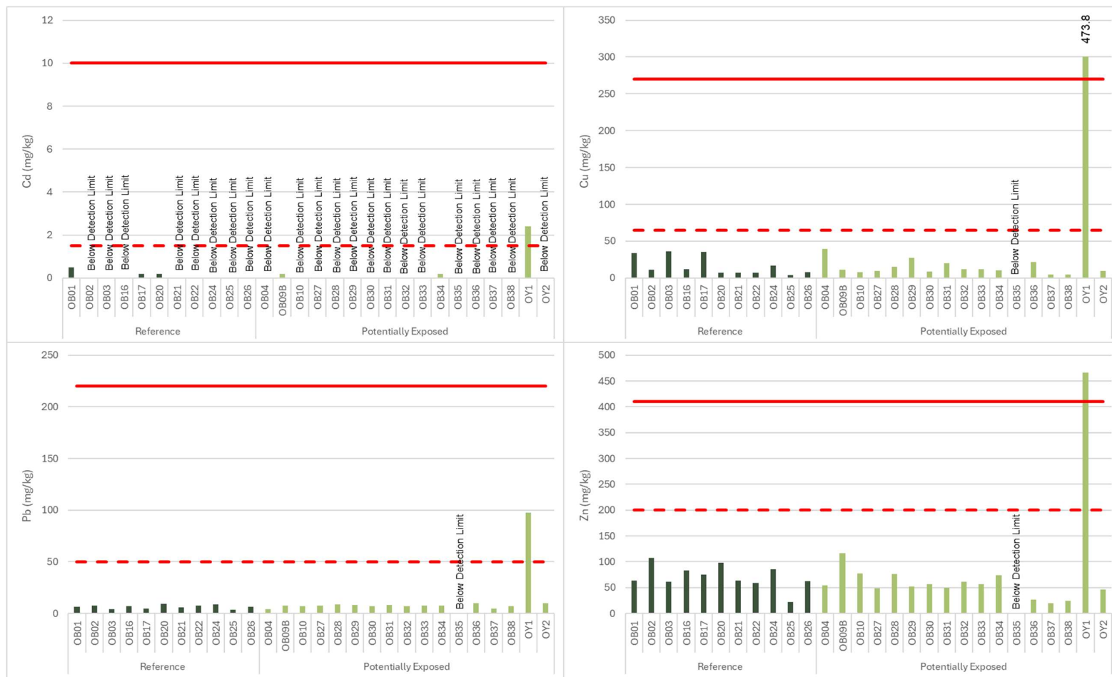
Figure 7. Concentration of metals within sediments (mg/kg dry weight), showing plots for Cd, Cu, Pb and Zn in comparison to DGV (broken line) and GV-High (solid line).
