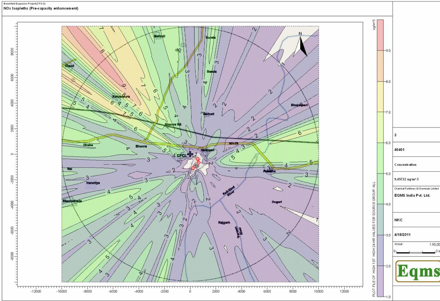
Figure 2.4 : NOx Isoleths (Initial Assessment)
