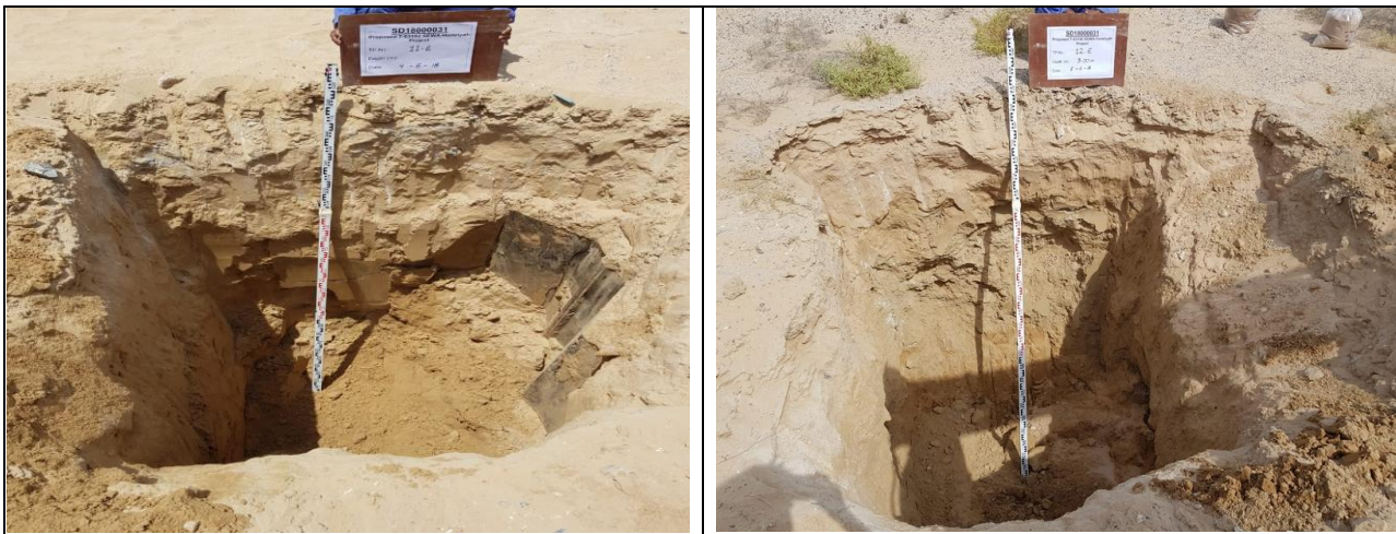
Figure 6: Typical Photographs during Trial Pit Excavation
