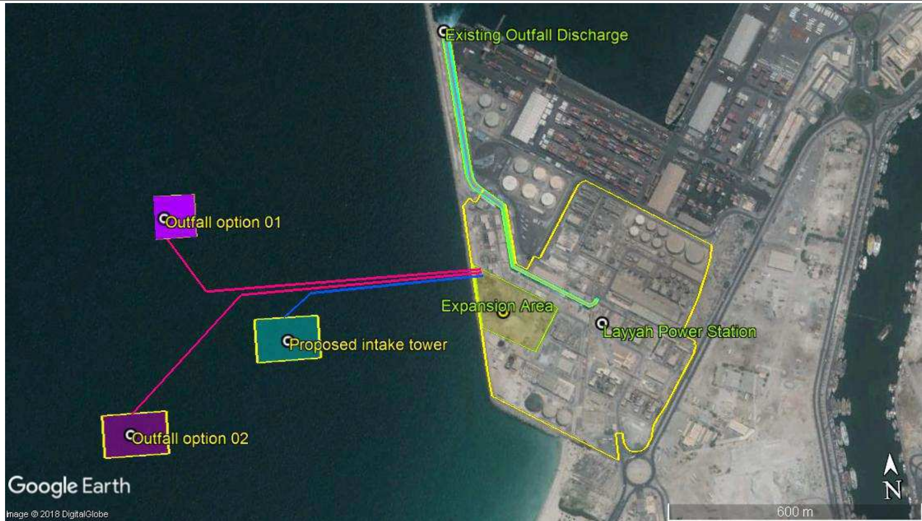
Figure 3 - Google Image showing the project site with proposed development with tentative intake and outfall locations
