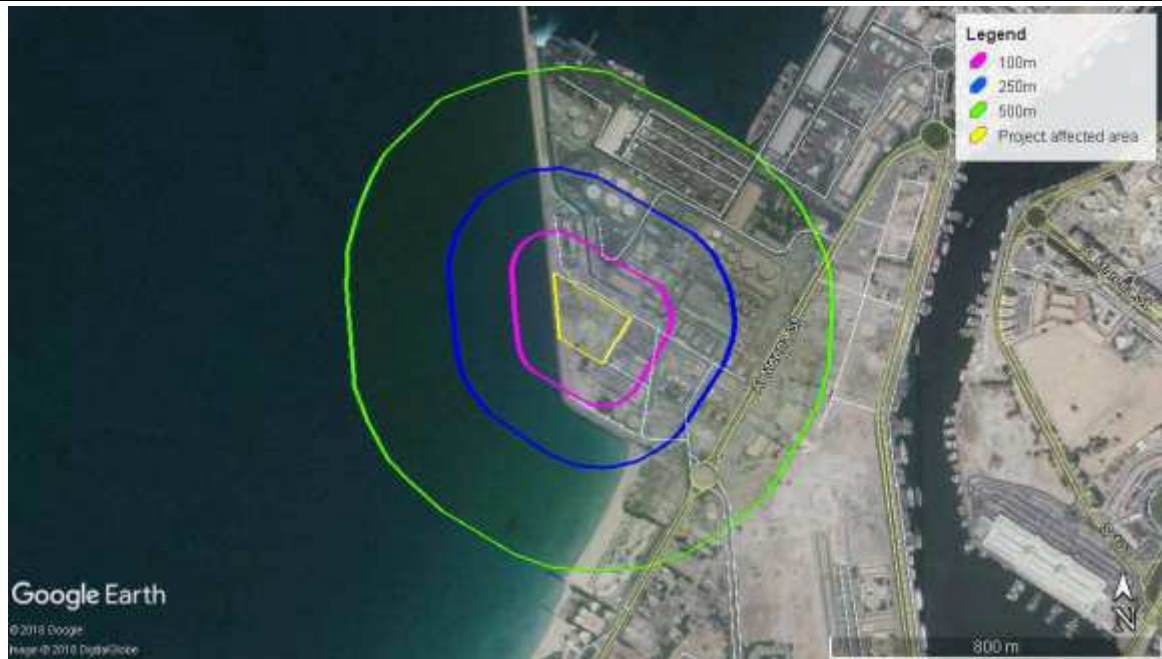
Figure 40 – Construction dust buffers for main construction site
