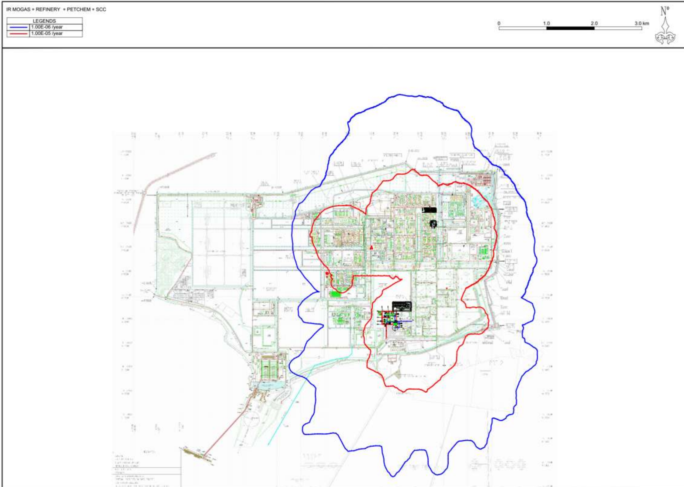
Figure D4: Cumulative Contour for EURO MOGAS Units, Olefins Storage Tankages, Refinery & Cracker Complex and Petrochemical Complex
