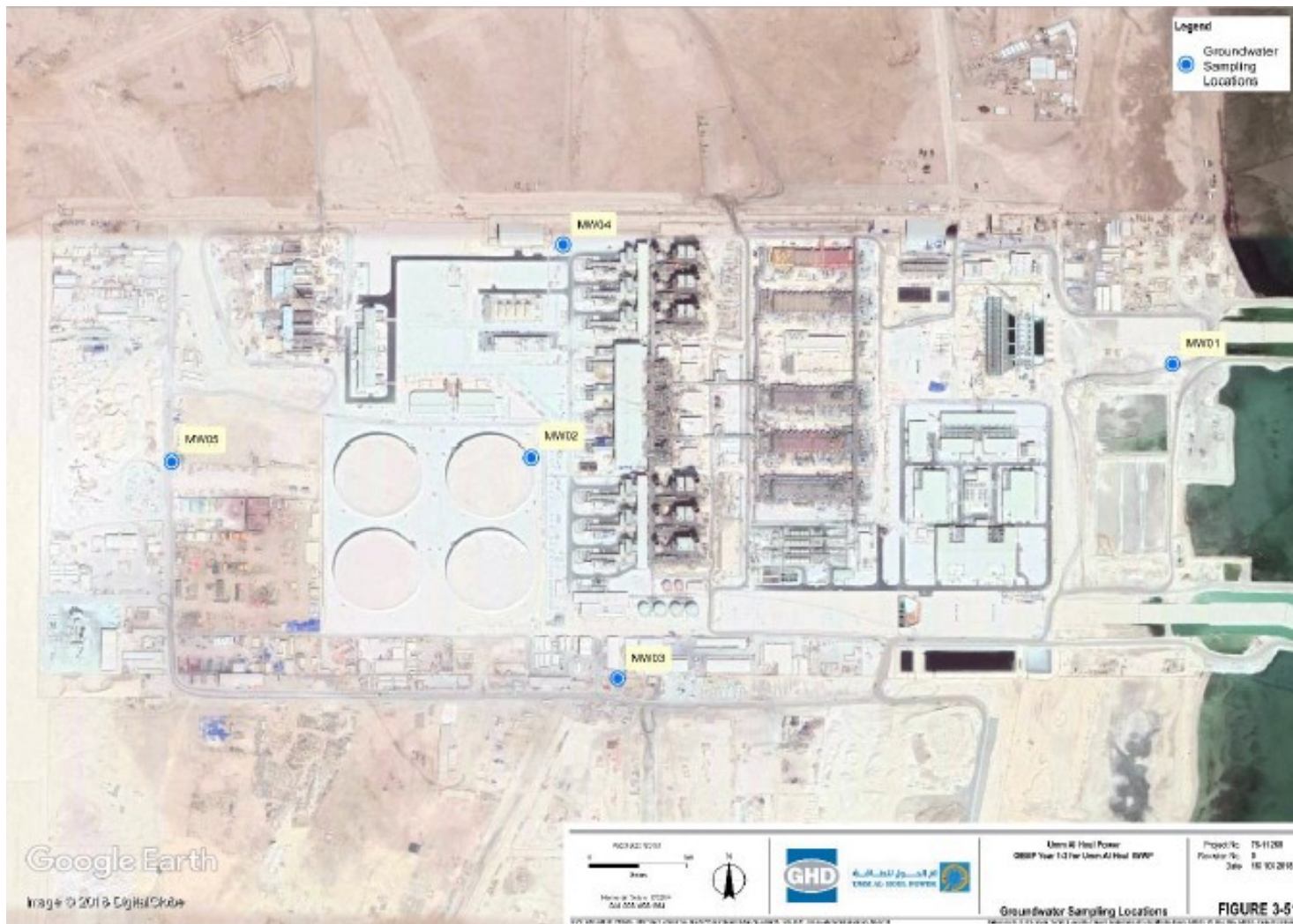
Figure 8-2: Locations of quarterly groundwater monitoring stations
