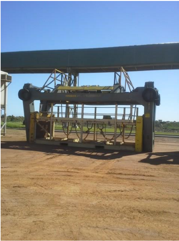
Figure 10: Rotating mechanism used during ship loading
