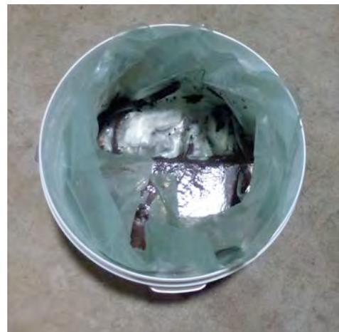
**PLATE 2:** Sub-sampling [tailings-slurry-water](#) and [tailings-solids](#) for testing.
