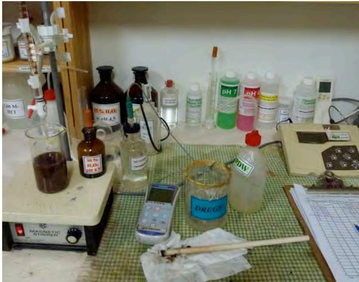
**PLATE 3:** Acid-Neutralisation-Capacity (ANC) testing.
