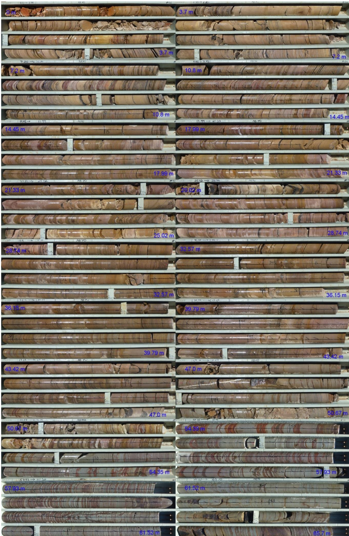
Figure 5-4: Diamond drill AB70 core images (0 to 65.7 mbgl) within northern part of deposit area (SWL in area ranges from 37 to 38 mbgl).
