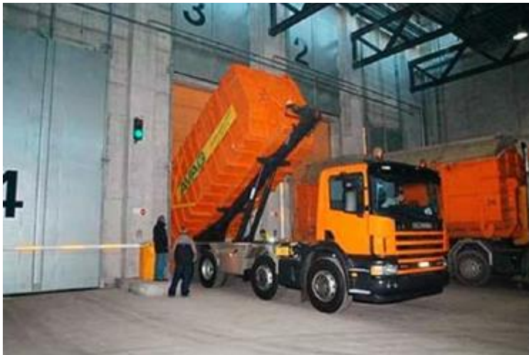
Figure 4-26 A typical waste delivery truck tipping off the waste into tipping bay
