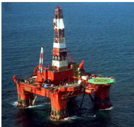
a) Semi-submersible MODU (source: Petro.No 2017, Maritime Connector 2017)
