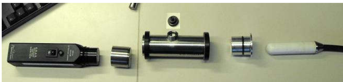
Figure 6. Split view of (left) a GRAS pistonphone calibrator, (middle) adaptors, and (right) a hydrophone.
