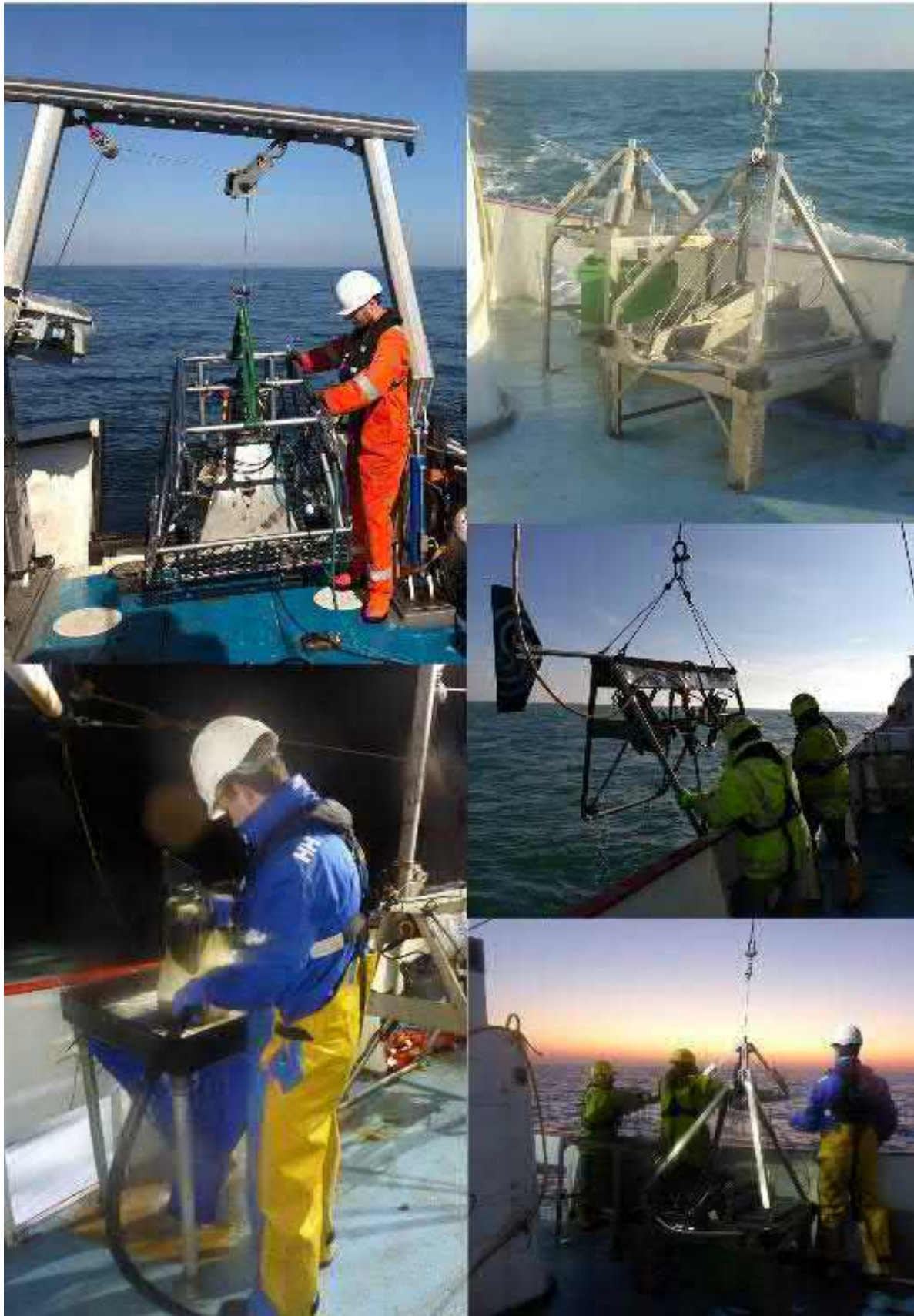
Plate 2. Top left: Deployment of freshwater housing camera system aboard Seren Las . Bottom left: Sieving of macrobenthic sample. Top right: Day and 0.1m 2 mini-Hamon grabs on deck. Middle right: Camera frame being deployed by Environmental Scientist. Bottom right: Deployment of 0.1m 2 Day grab using ships starboard side crane.
