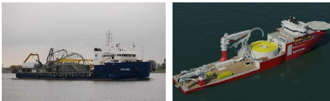
Figuur 4-25: Kabellegger (Links: de Topaz Installer, rechts: de Aker Connector)
