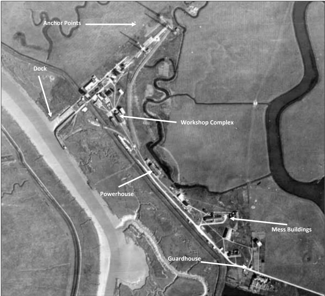
1946 aerial imagery of the Yantlet firing point main complex, situated approximately 1.5km west of the western endpoint of the study area. Railway firing points (and the rail tracks leading up to them), gun emplacements and gantry paths can all be identified surrounding this image.
