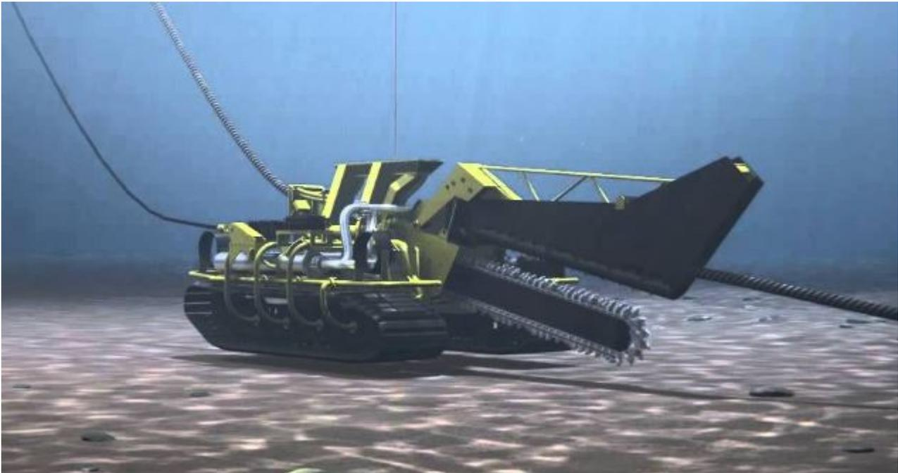
When using this method, the trench should remain as narrow as possible and the trench is typically filled in by the natural movement of the seabed materials. In hard soils where rock trenching is necessary, a reduced burial depth is typically acceptable considering reduced anchor and trawler penetrations into the seabed.
