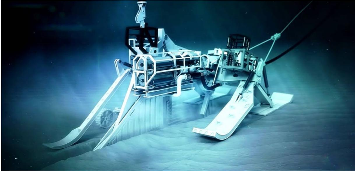
For burial to depths considerably deeper than 2-3metres below seafloor, for example, up to 10meters into sands, in areas closer to shore, the Vertical Injector (VI) technique is recommended. Machines like the one shown in Figure 7-5 are designed for SLB operations.
