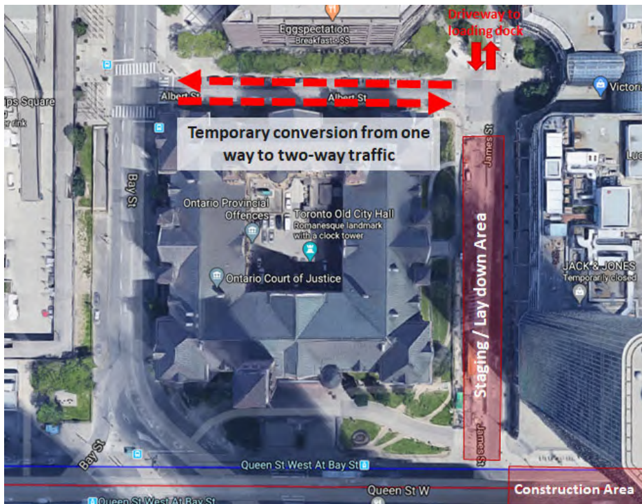
Figure 4-16: James Street Laydown | Access Impacts
