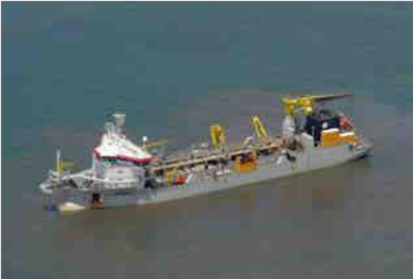
Figure 4-13 - Trailer Suction Hopper Dredger
