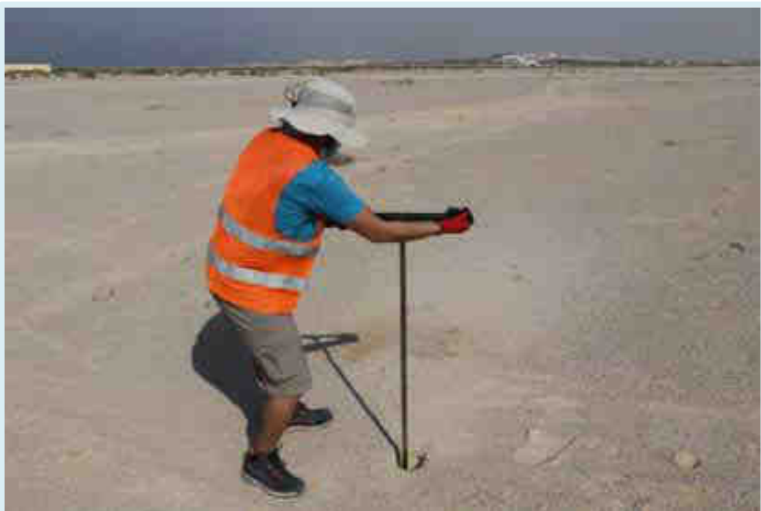
Plate 1: NEA Environmental Technician using soil augur on site wearing PPE
