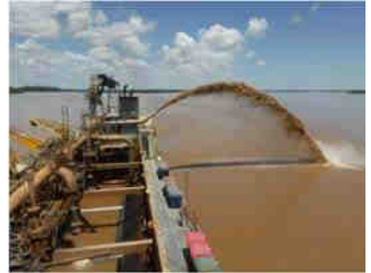
Trailing Suction Hopper Dredger (TSHD)
