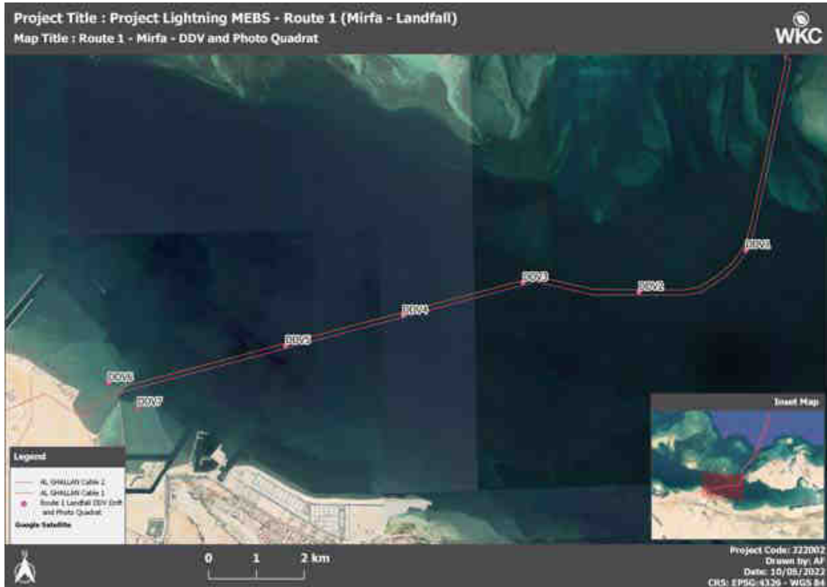
Figure 6-2 – DDV Survey sites at Route 1 (Mirfa) Landfall
