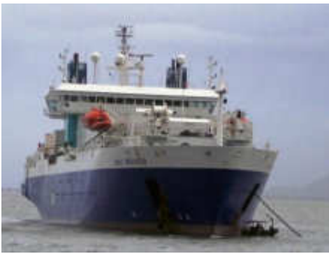
Cable Laying Vessel (source : Nathan Sandel)
