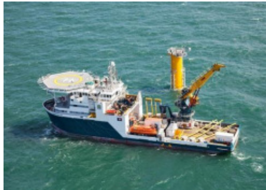
Diving support Vessel (source : Liftra)
