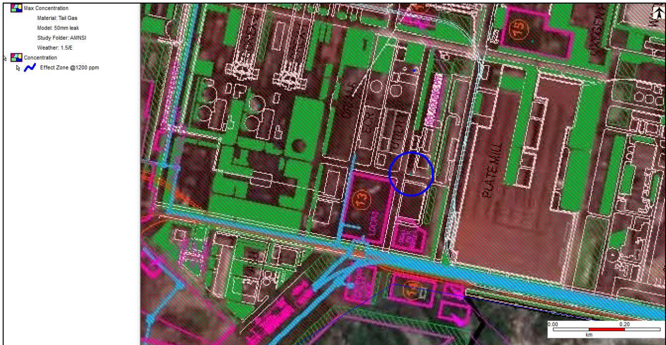
Figure 7-13: Max concentration effect distance contour due to catastrophic rupture of Tail Gas holder at weather condition 1.5/E
