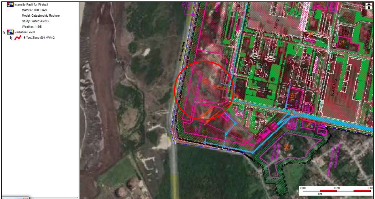
Figure 7-6: Flash fire effect distance contour due to catastrophic rupture of BOF Gas holder at weather condition 4/D
