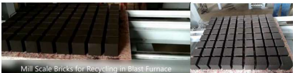
Figure 4-30: Mill scale briquettes for recycling in blast furnace.
