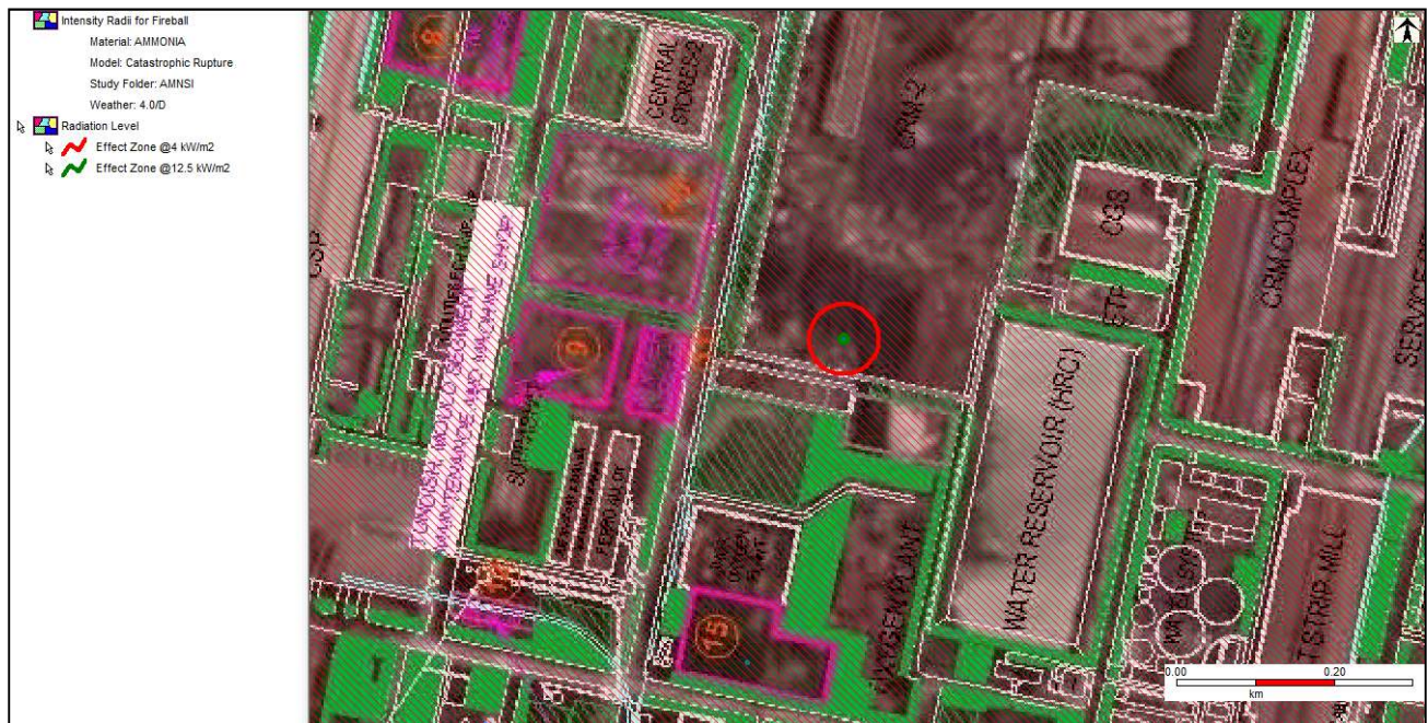
Figure 7-16: Fireball effect distance contour due to catastrophic rupture of Ammonia tank at weather condition 4/D
