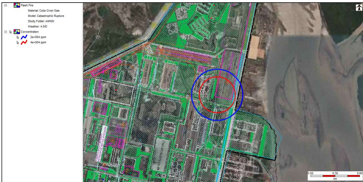
Figure 7-15: Flash fire effect distance contour due to catastrophic rupture of Coke Oven Gas Holder at weather condition 4/D
