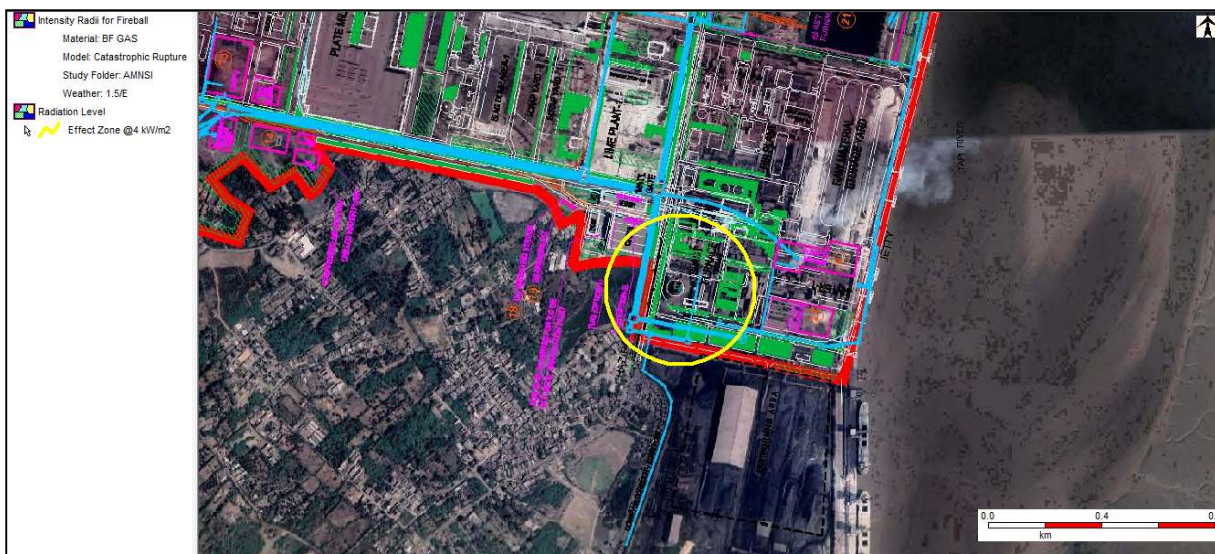
Figure 7-3: Flash fire effect distance contour due to catastrophic rupture of BF Gas holder at weather condition 4/D
