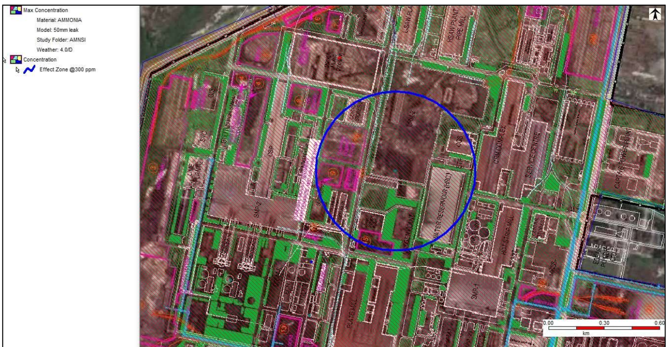
Figure 7-18: Max concentration effect distance contour due to catastrophic rupture of Ammonia at weather condition 4/D
