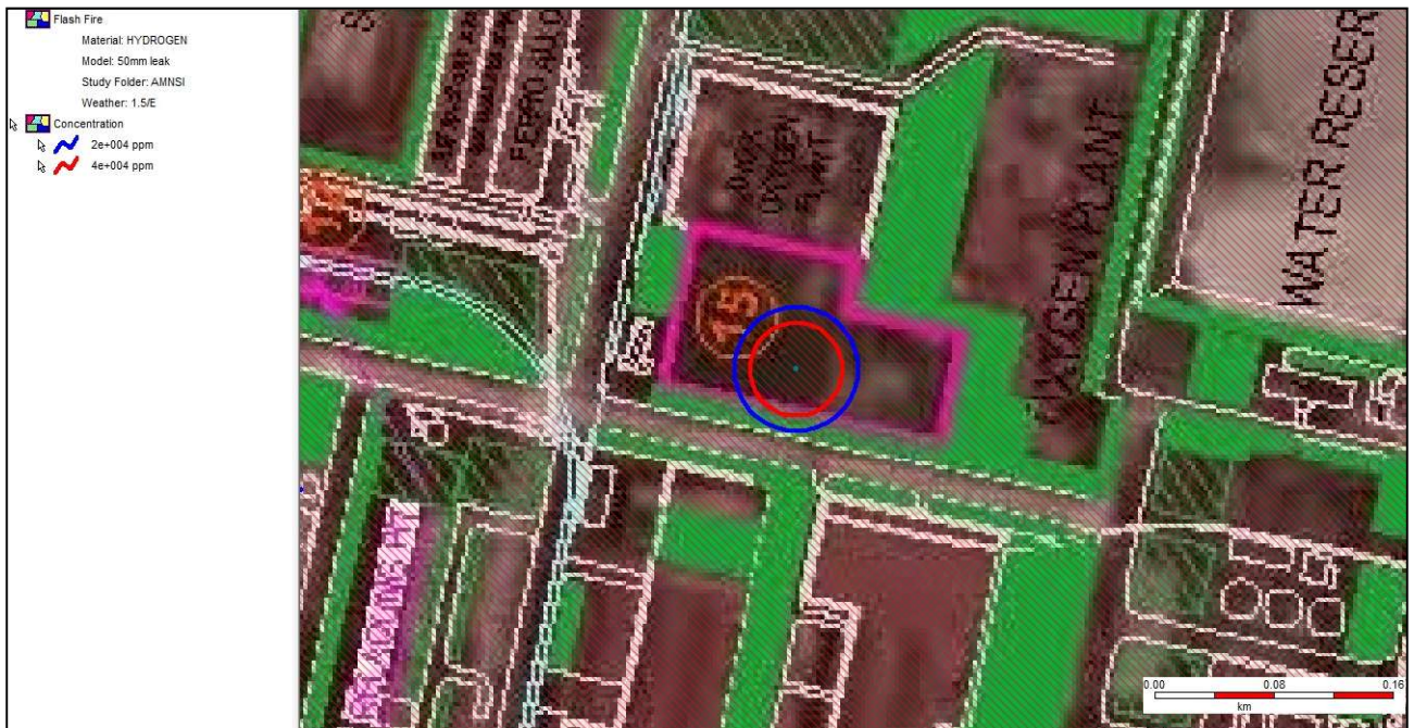
Figure 7-20: Flash fire effect distance contour due to catastrophic rupture of Hydrogen tank at weather condition 1.5/E
