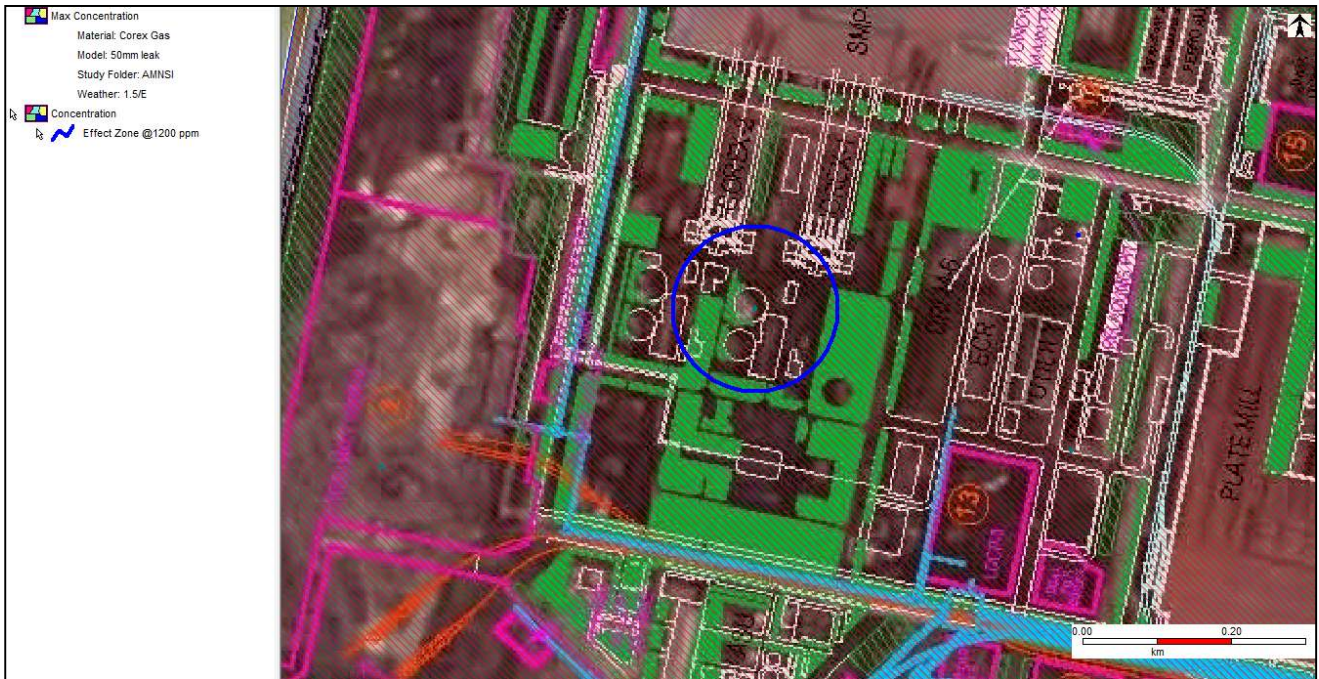
Figure 7-10: Max concentration effect distance contour due to catastrophic rupture of Corex Gas holder at weather condition 1.5/E
