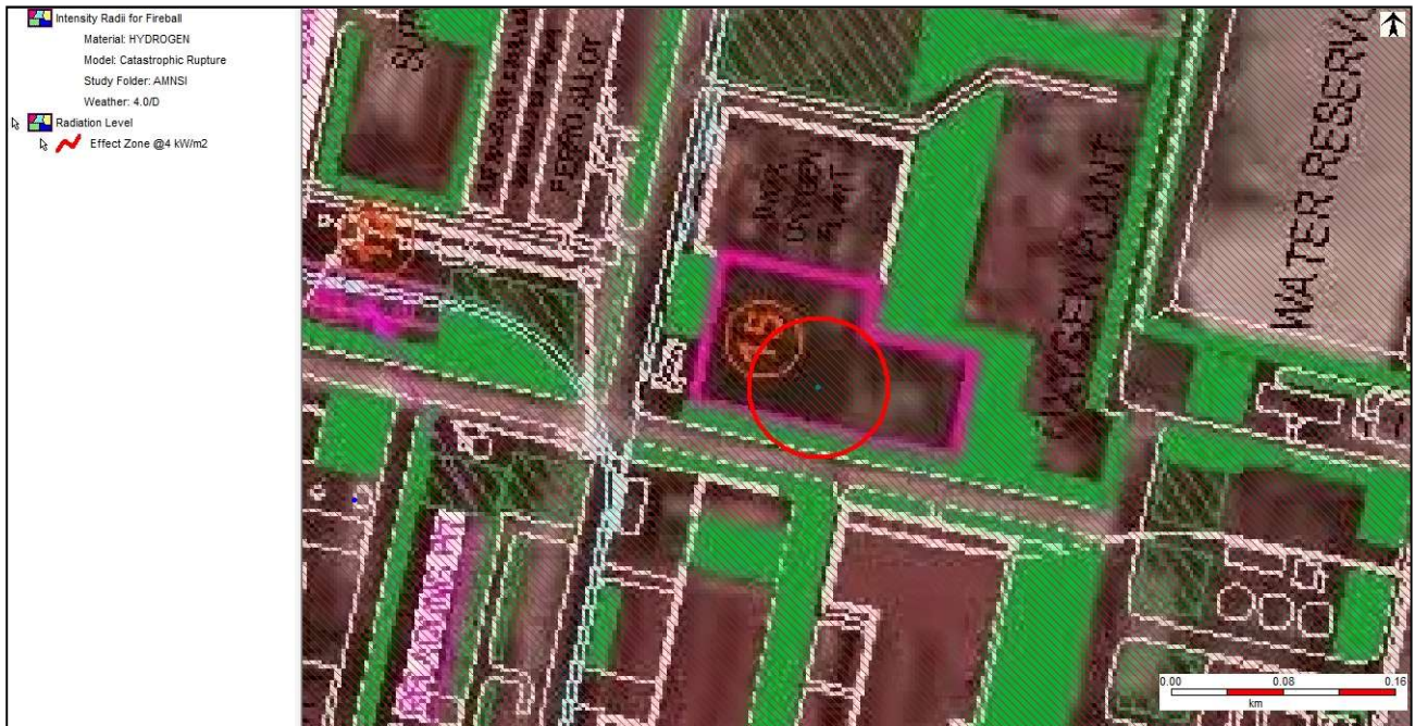
Figure 7-19: Fireball effect distance contour due to catastrophic rupture of Hydrogen tank at weather condition 4/D
