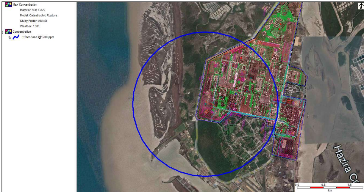
Figure 7-7: Max concentration effect distance contour due to catastrophic rupture of BOF Gas holder at weather condition 1.5/E
