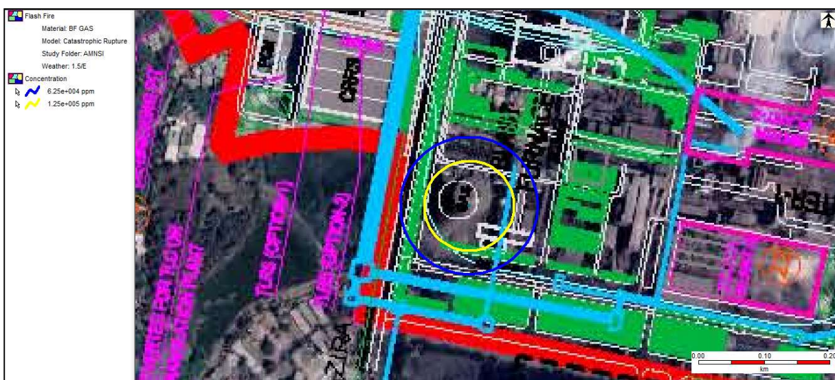
Figure 7-3: Flash fire effect distance contour due to catastrophic rupture of BF Gas holder at weather condition 4/D
