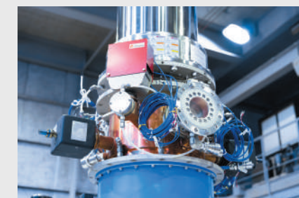
A gyrotron is a device that heats fuels such as tritium to a plasma state and uses microwaves to heat the plasma to over 100 million degrees Celsius, creating the high-temperature conditions necessary for fusion reactions.
