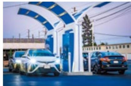
Two types of hydrogen fuel, 70MPa for passenger vehicles and 35MPa for heavy vehicles, are available.
