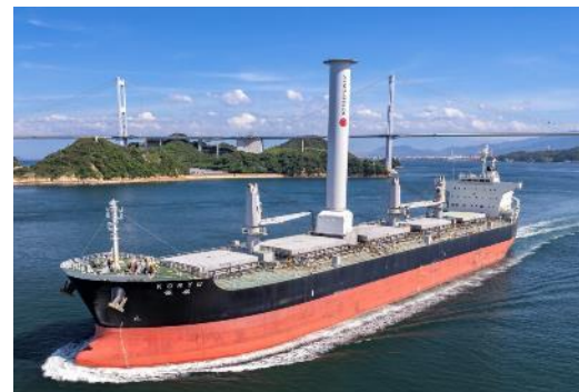
M/V KORYU, a copper concentrates and sulphuric acid carrier equipped with a Rotor Sail, a wind-assisted propulsion system, on its deck (Source: Japan Marine Co., Ltd. website)
