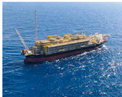
An FPSO vessel of the same type used in the project. (provided by MODEC, Inc.)
