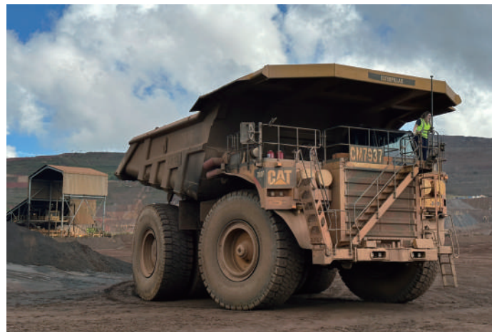
Huge dump truck with a payload capacity of 240 tons, which is used in the mine
