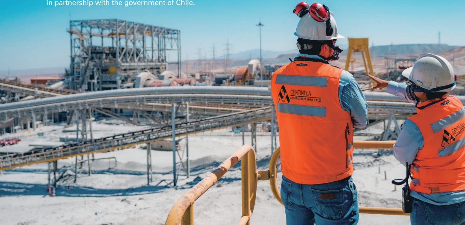
The ore beneficiation plant which crushes ore from the Centinela copper mine in northern Chile, and separates and recovers copper.
