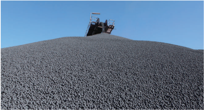
Pellets are spheres with a diameter of 1 to 3 centimeters made from processed iron ore.
