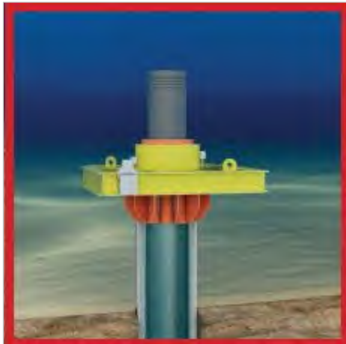
Figure 4-2 Diagram of wellhead structure representative of the Thebe-1 wellhead on the seabed
