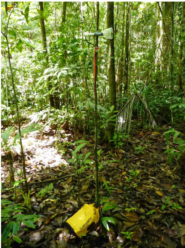
Plate 3 A Pettersson Elektronik D500X bat detector in a waterproof bag, with a microphone on a 3-meter extension cable and protected from rain in a plastic funnel.
