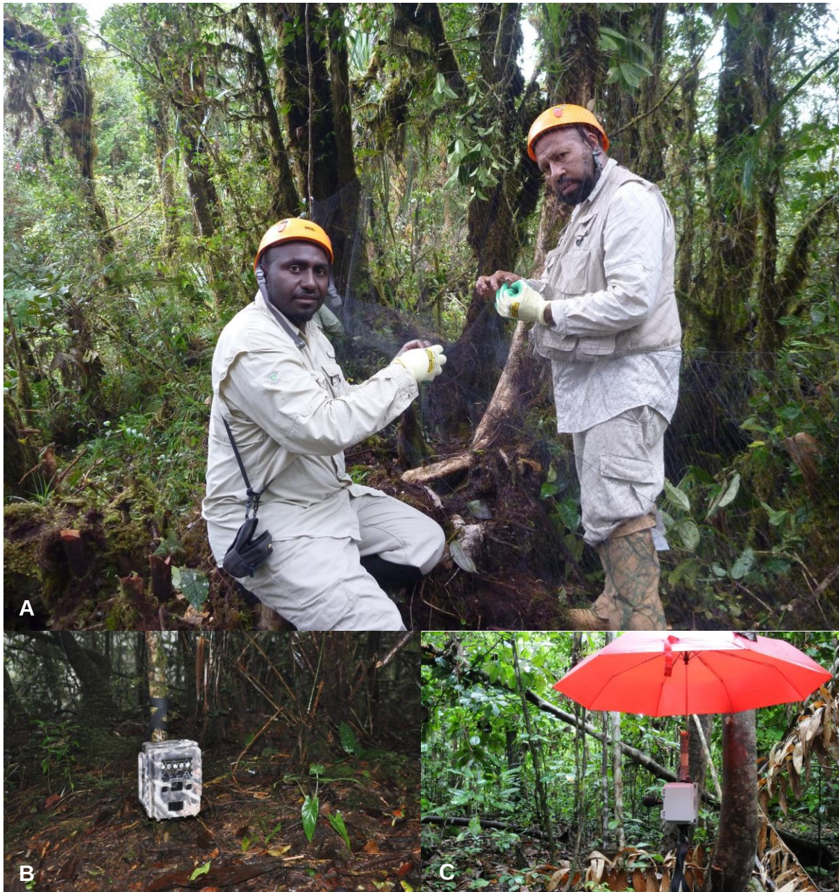
Plate 1 Equipment used during bird surveys: (A) mist net; (B) camera trap; (C) automated sound recorder.
