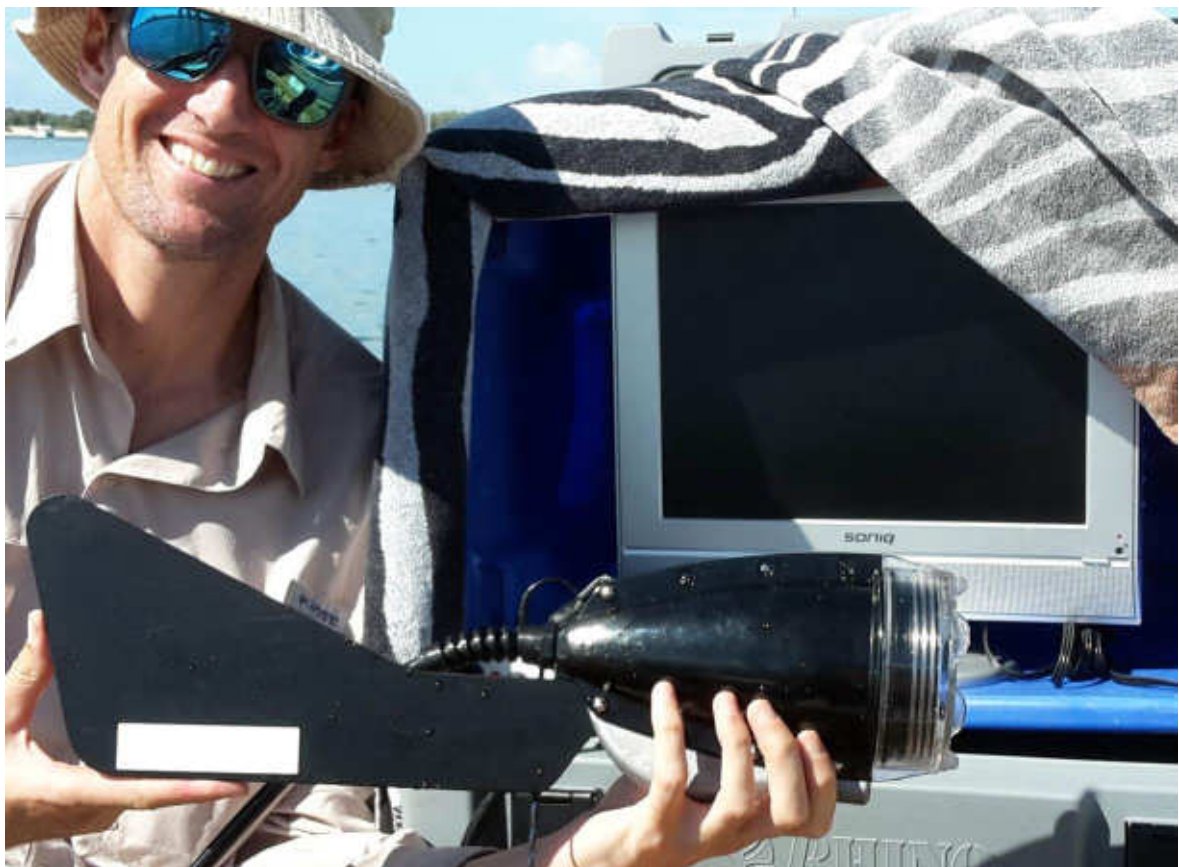
Figure 5-5 Drop Camera Used for Validation
