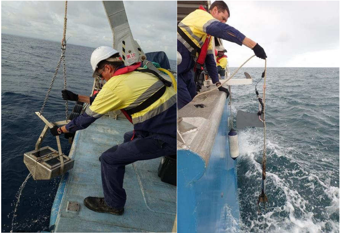
Figure 5-4 Field Survey Techniques: benthic macroinvertebrate sampling using Van Veen grab (left) and deployment of drop camera for validation (right)
