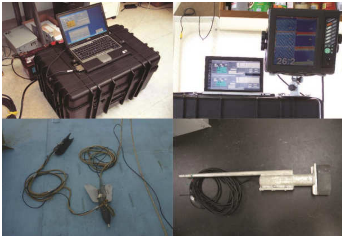
Figure 5-6 Acoustic Survey Equipment: Single-beam Acoustic Capture Hardware (Top Left); Single-Beam Acoustic Downscan (Top Right); Sidescan Towfish, Bomb, and Tow-line (Lower Left); 200 kHz transducer (Lower Right)
