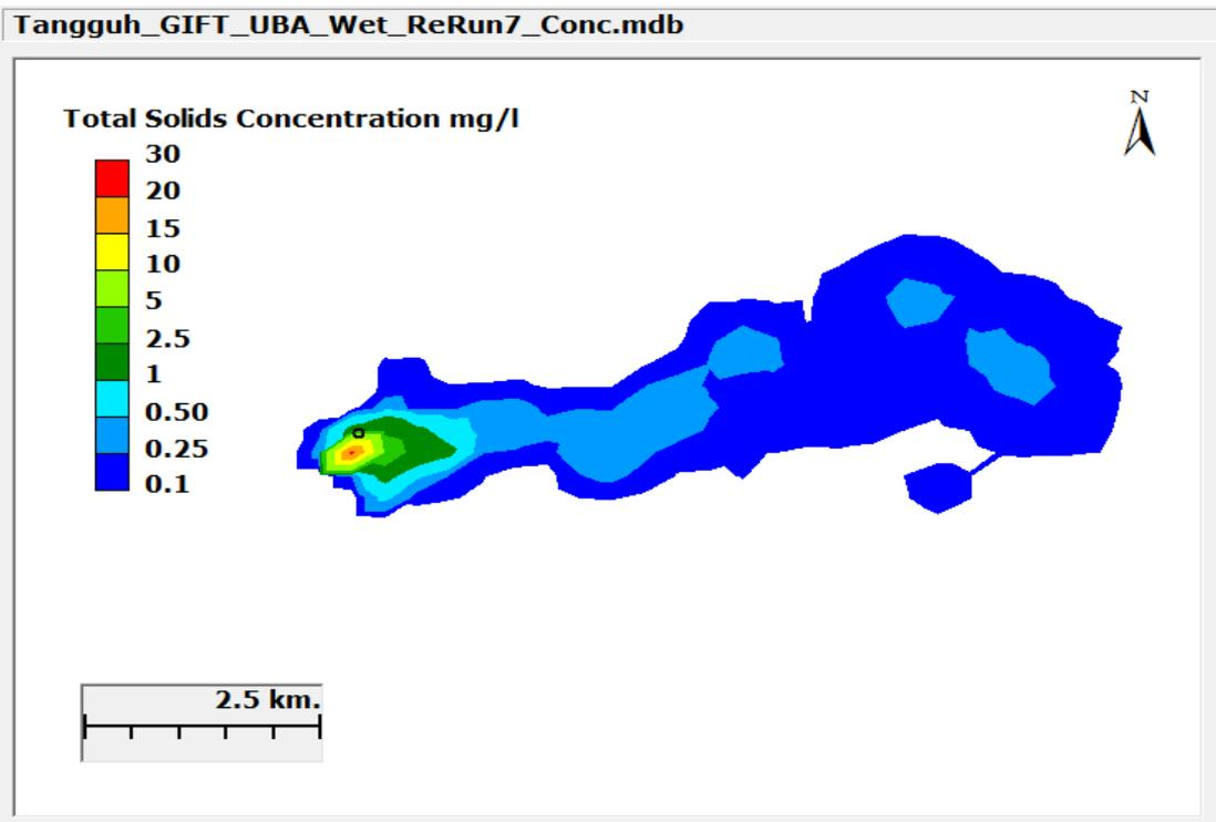
Figure III-10 Maximum Increase in TSS Concentration During Drilling in UBA During the Wet Season
