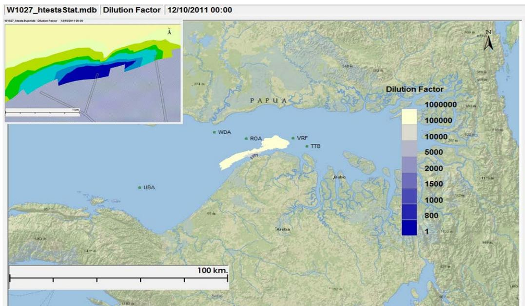
**Figure III-27** Minimum Dilution Factor Contour Plot of the Combined Hydrotest Water and Comingled Wastewater at the LNG Jetty 2 during the Wet season
