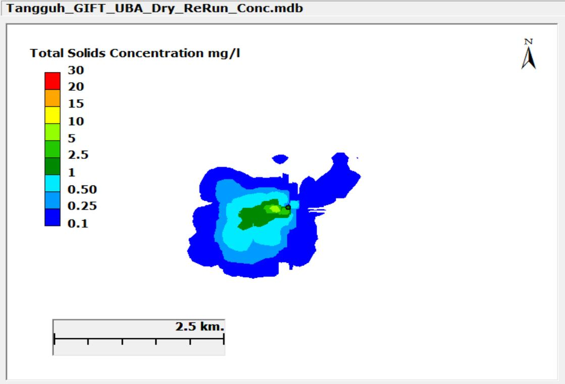
Figure III-9 Maximum Increase in TSS Concentration During Drilling in UBA During the Dry Season
