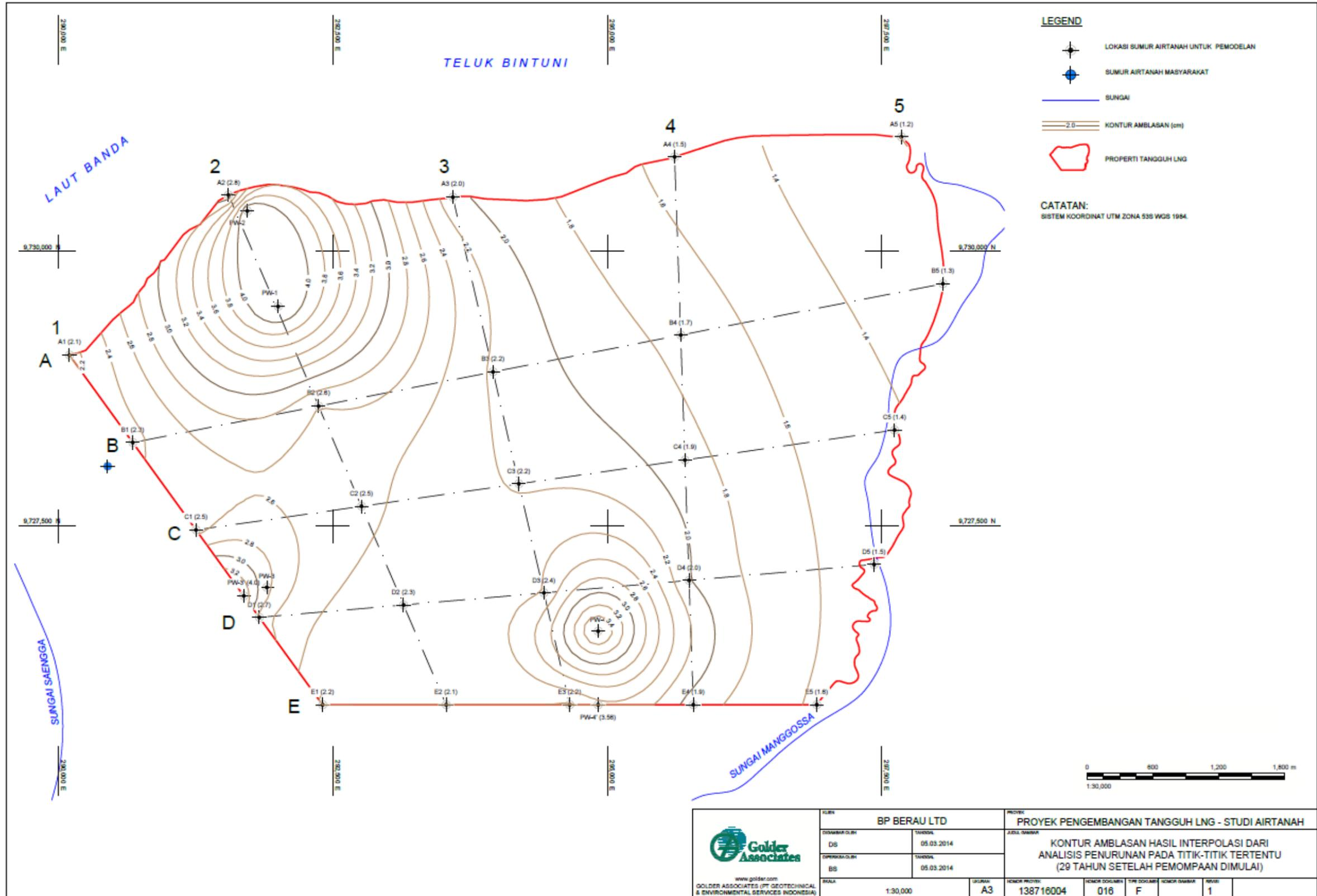
Figure III-46 Subsidence Contour from Interpolation of Subsidence Analysis at Specific Points (29 Years after Pumping Commenced)
