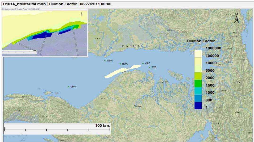
**Figure III-26** Minimum Dilution Factor Contour Plot of the Combined Hydrotest Water and Comingled Wastewater at the LNG Jetty 2 during the Dry Season
