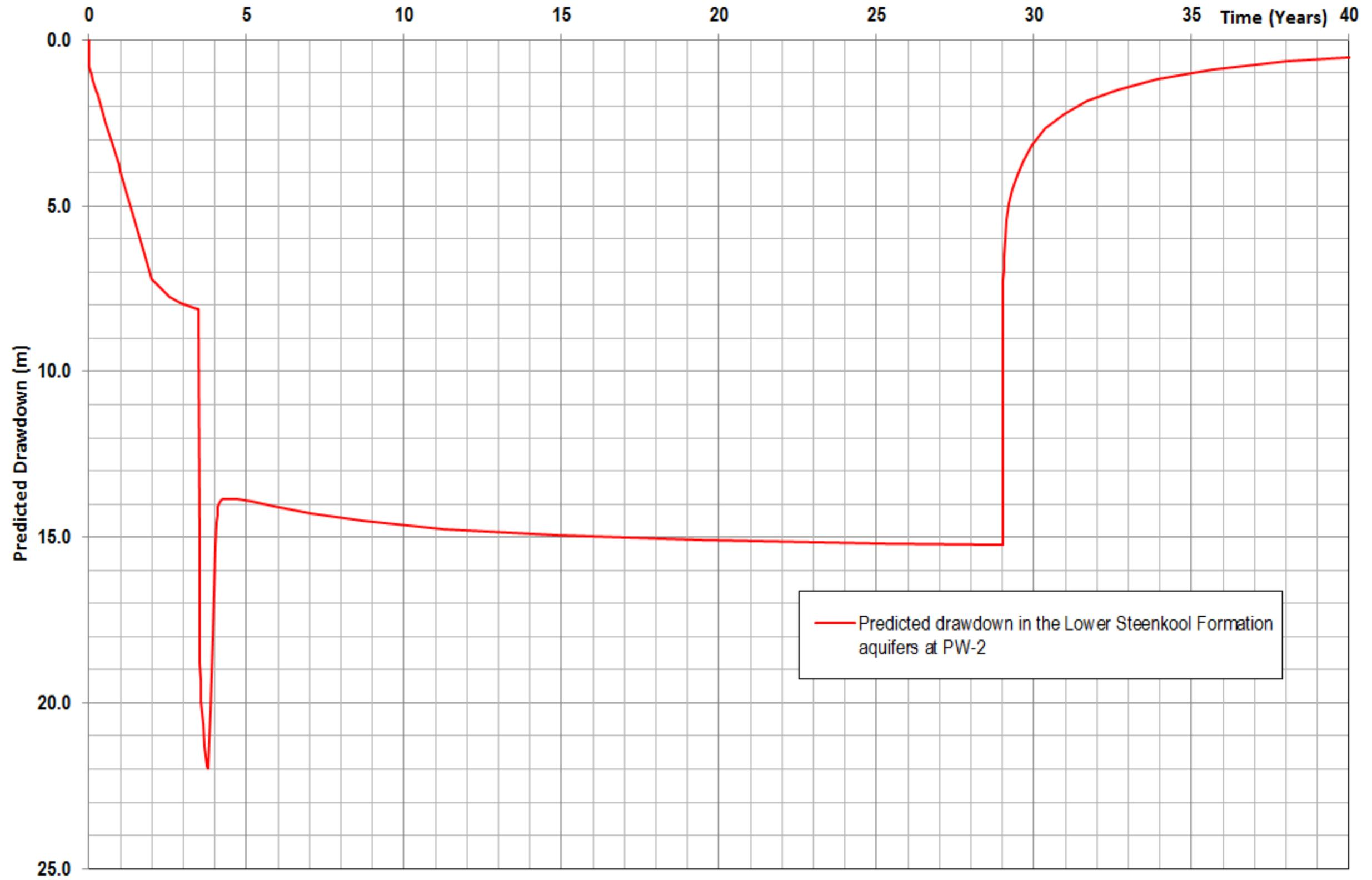
Figure III-43 Predicted Drawdown and Rebound of Water Level in Lower Steenkool Formation Aquifer at PW-2
