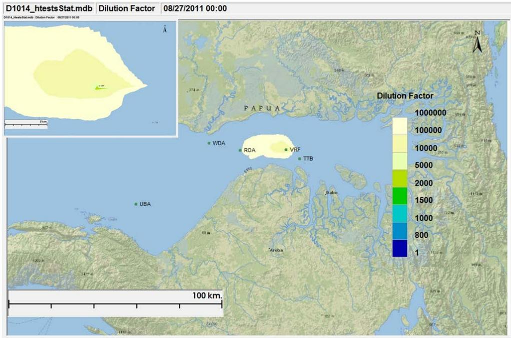
**Figure III-20 Minimum Dilution Factor Contour Plot of Hydrotest Water Discharge at VRF during the Dry Season**
