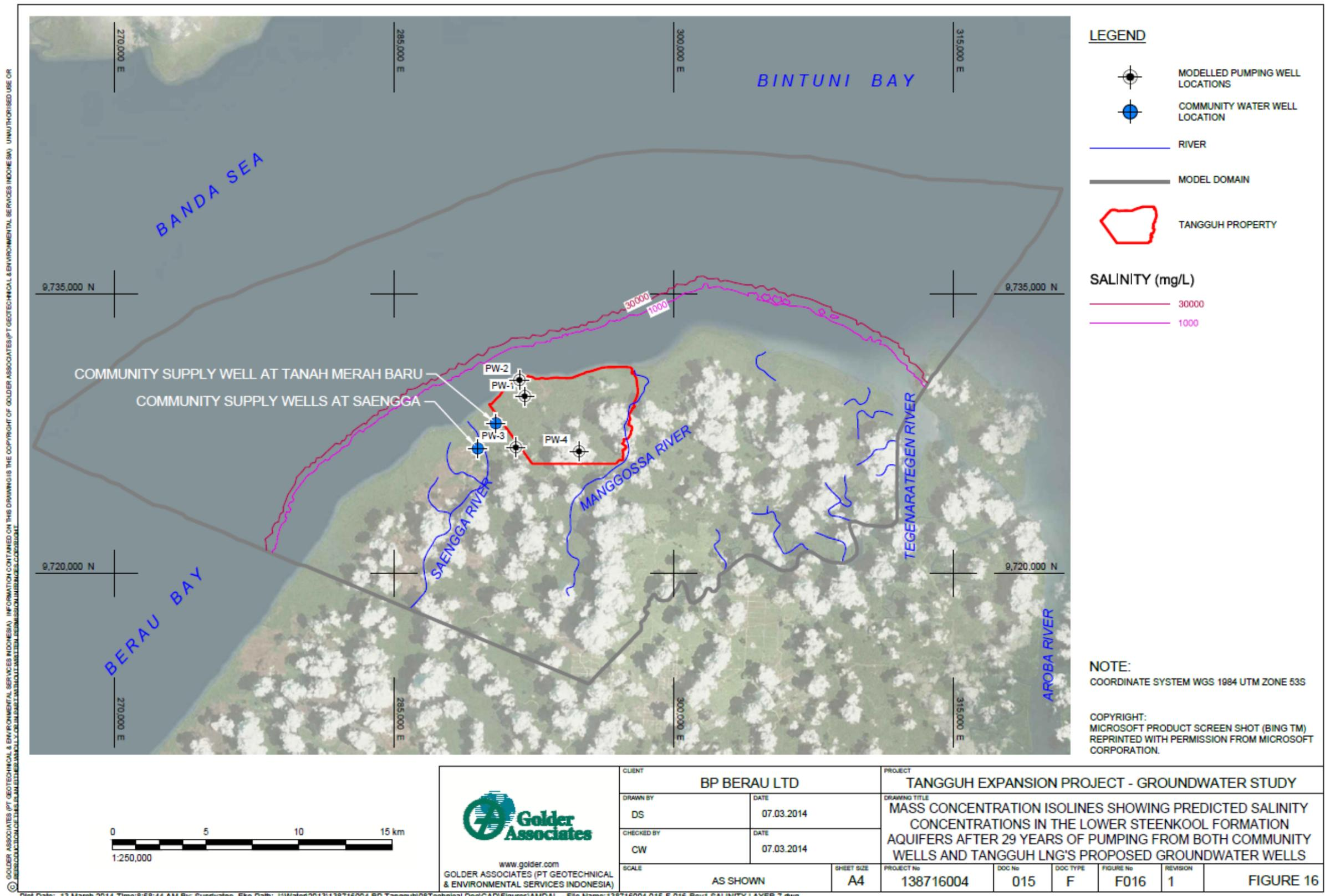
**Figure III-44** Mass Concentration Isolines showing Predicted Salinity Concentrations in Steenkool Formation Aquifer after 29 years of Pumping from Community Wells and the Proposed Groundwater Wells of the Tangguh LNG
