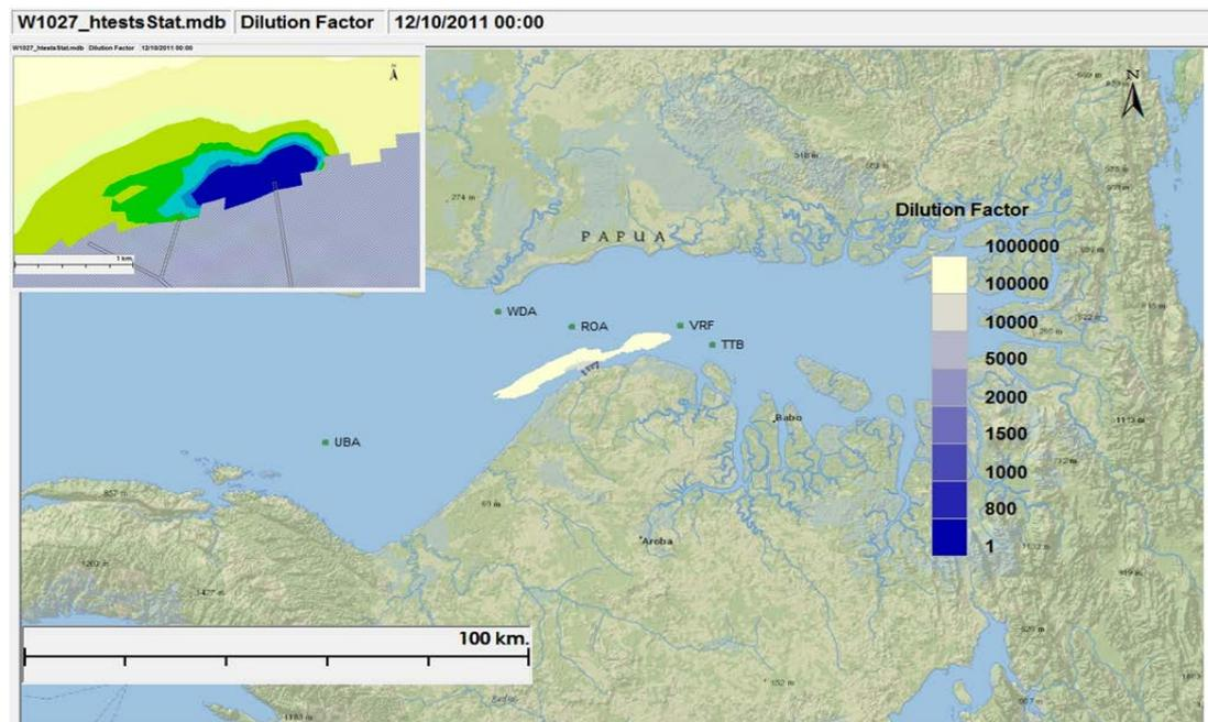
**Figure III-25** Minimum Dilution Factor Contour Plot of the Combined Hydrotest Water and Comingled Wastewater Discharge at the LNG Jetty 1 during the Wet season
