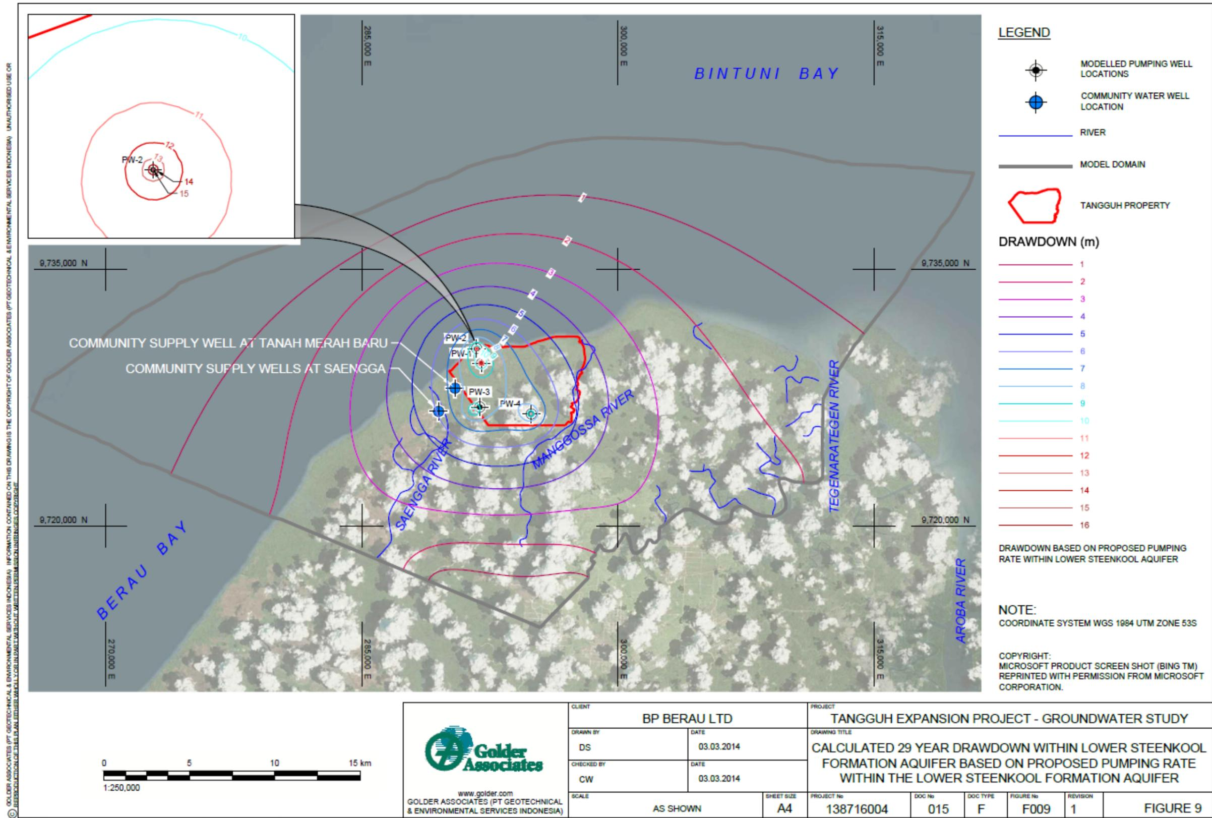
Figure III-39 Modeling of Water Table for 29 Years in the Lower Steenkool Formation Aquifer based on Proposed Pumping Rate
