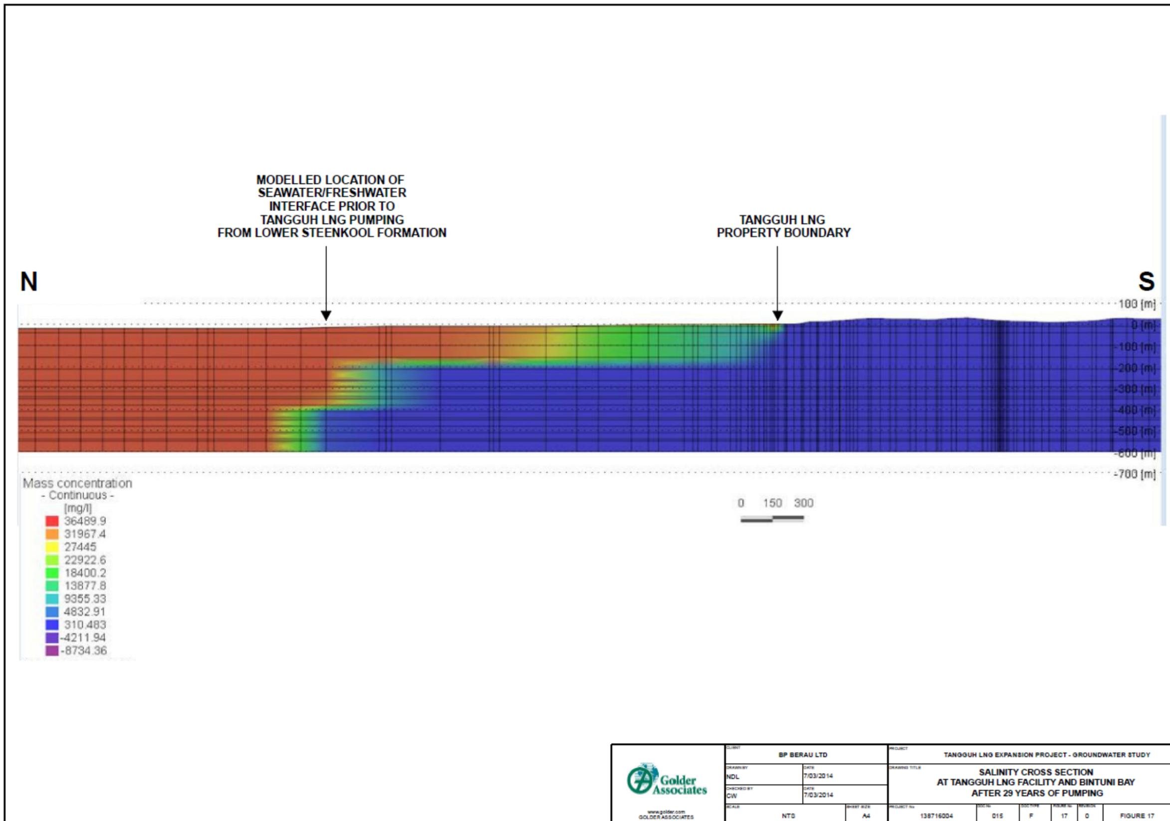
Figure III-45 Salinity Cross Section at the Tangguh LNG Facility and Bintuni Bay after 29 years of Pumping
