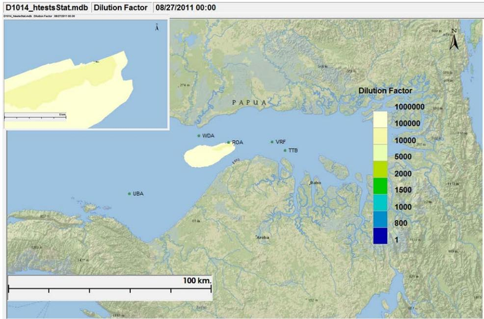
Figure III-16 Minimum Dilution Factor Contour Plot of Hydrotest Water Discharge at ROA during the Dry Season
