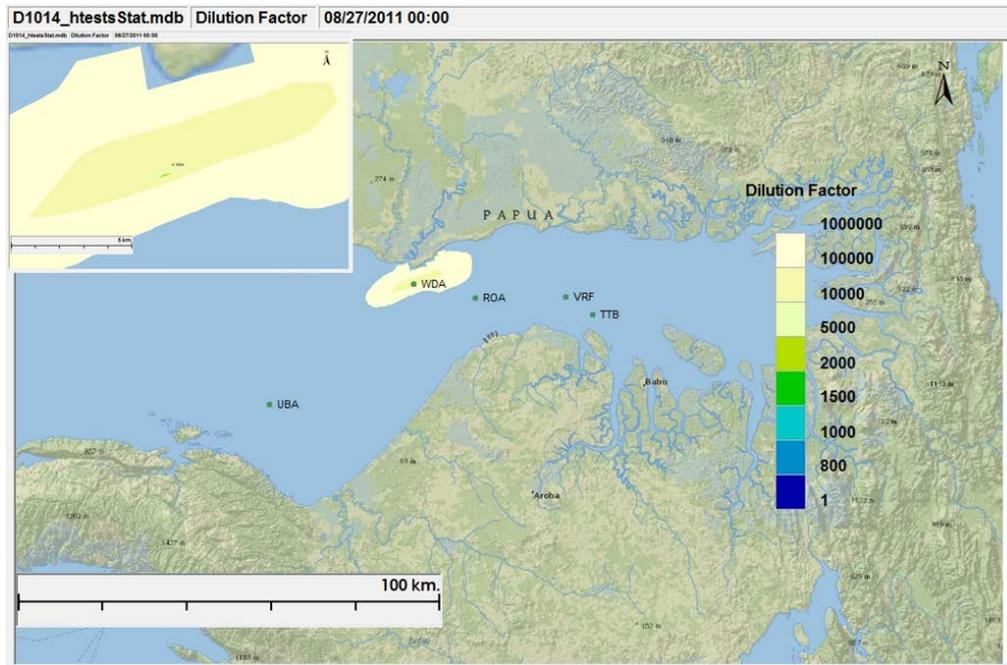
Figure III-18 Minimum Dilution Factor Contour Plot of Hydrotest Water Discharge at WDA during the Dry Season
