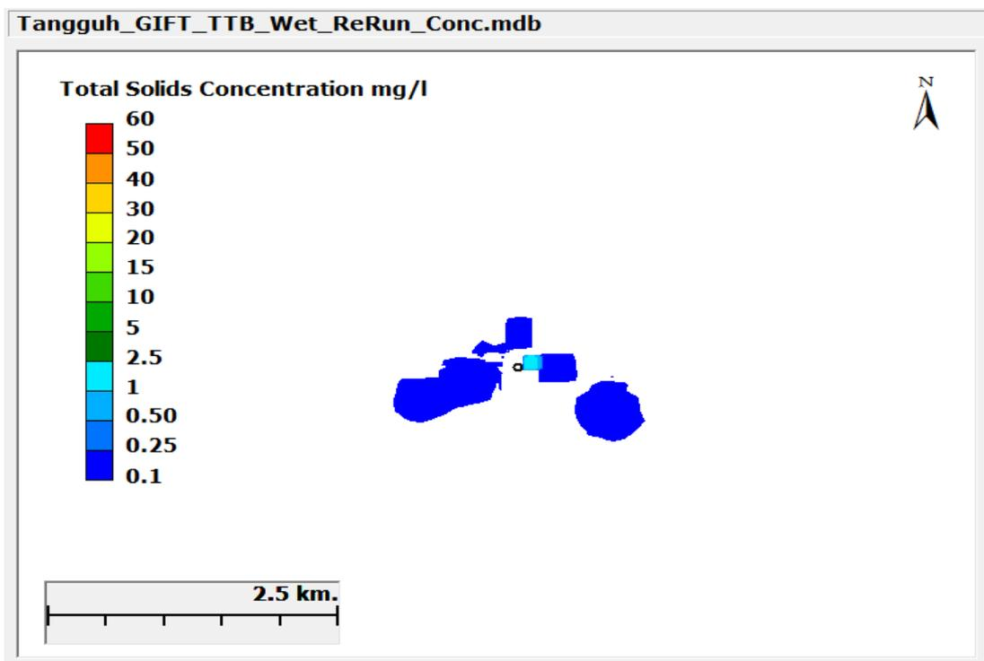
Figure III-6 Maximum Increase in TSS Concentrations During Drilling in TTB During the Wet Season
