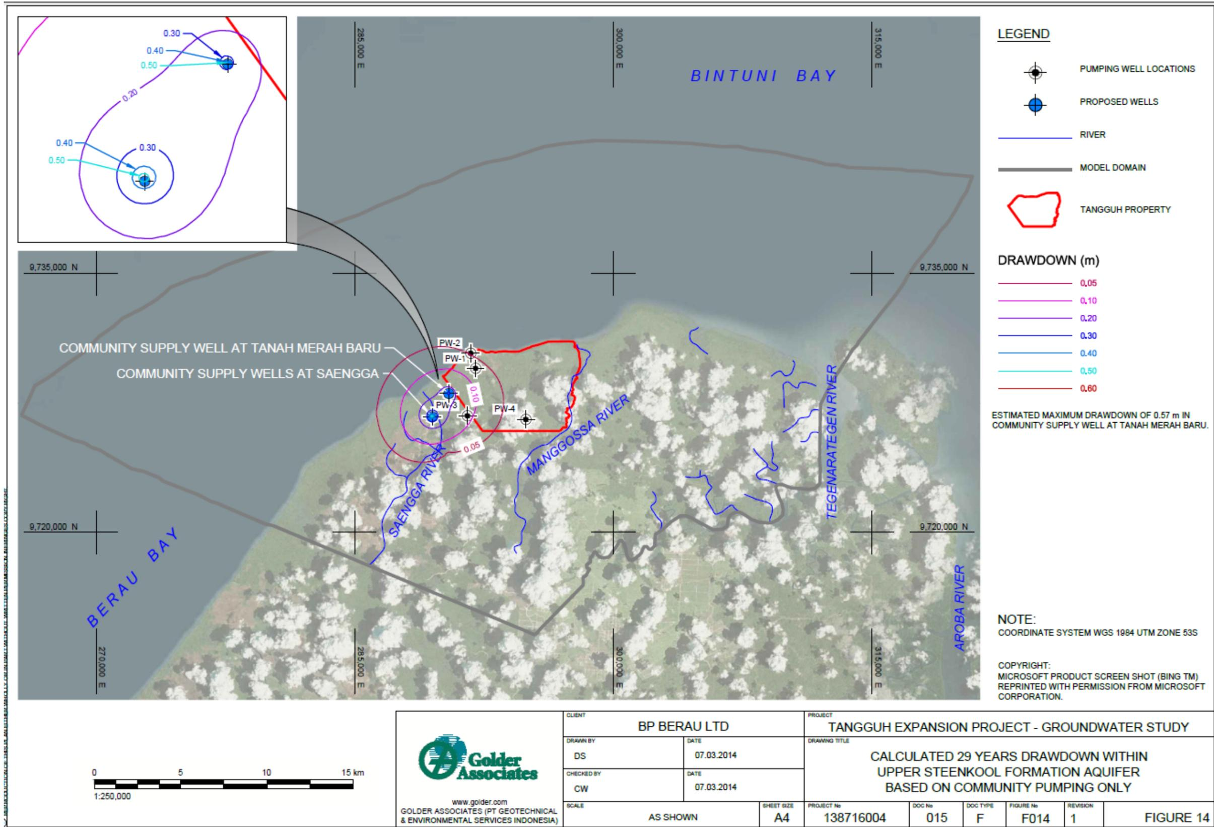
Figure III-40 Modeling of Water Table for 29 Year in the Upper Steenkool Formation Aquifer based on Community Wells Pumping at Tanah Merah Baru and Saengga
