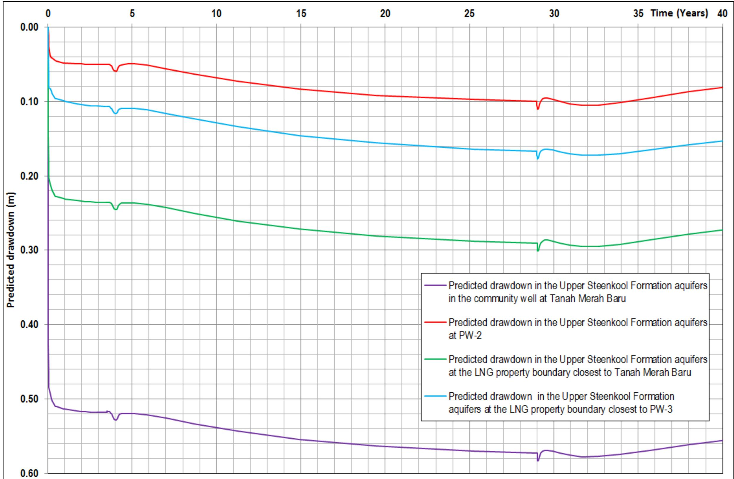
Figure III-42 Predicted Drawdown and Rebound of Water Level in Upper Steenkool Formation Aquifer at PW-2, Community Well at Tanah Merah Baru, at the Boundary Area of the Tangguh LNG nearest to PW-3 and the Boundary Area of the Tangguh nearest to Tanah Merah Baru Village
