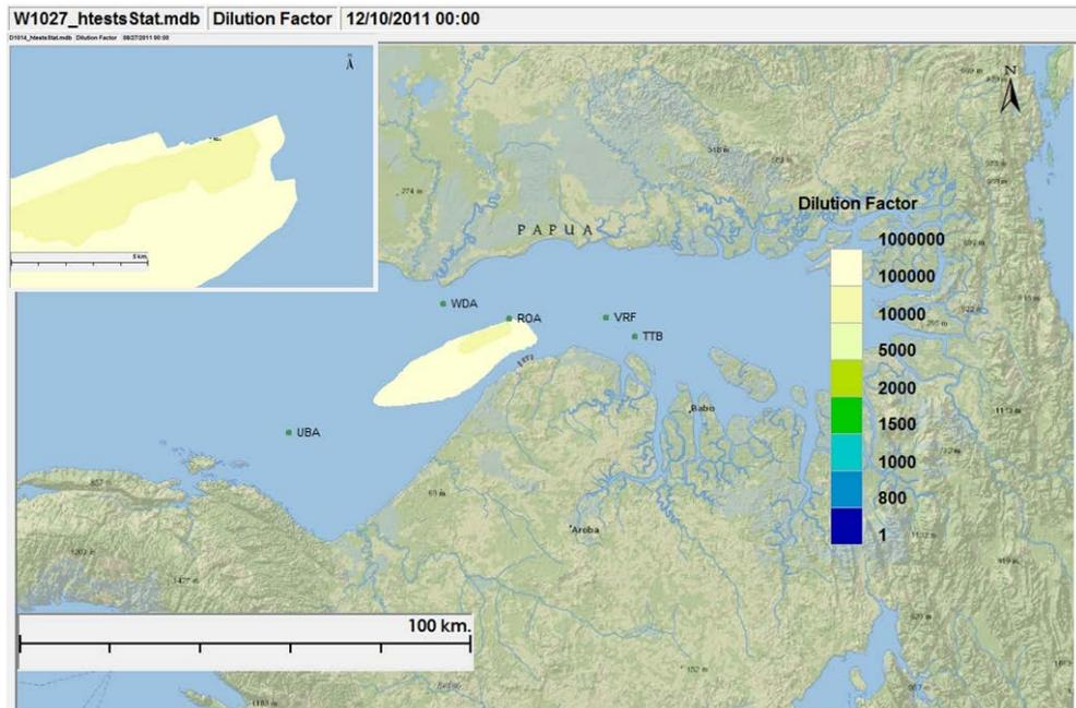
Figure III-17 Minimum Dilution Factor Contour Plot of Hydrotest Water Discharge at ROA during the Wet season
