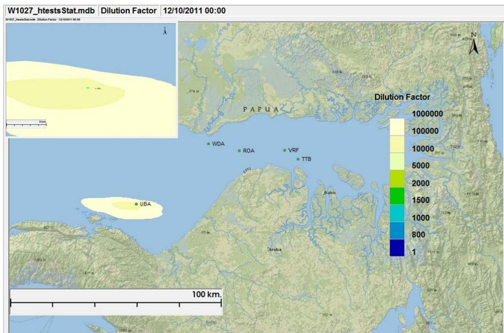
Figure III-23 Minimum Dilution Factor Contour Plot of Hydrotest Water Discharge at UBA during the Wet season
