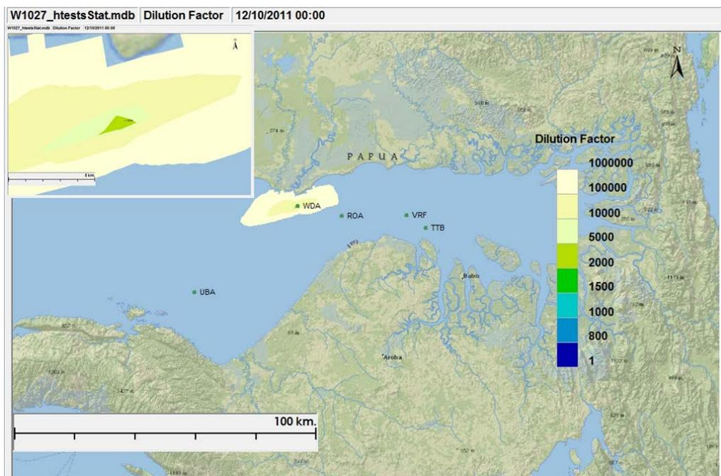
Figure III-19 Minimum Dilution Factor Contour Plot of Hydrotest Water Discharge at WDA during the Wet season
