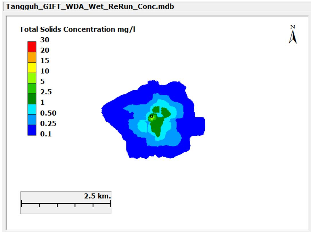
**Figure III-8 Maximum Increase in TSS Concentration During Drilling in WDA During the Wet season**
