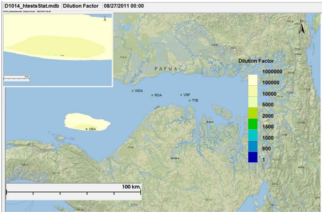
Figure III-22 Minimum Dilution Factor Contour Plot of Hydrotest Water Discharge at UBA during the Dry Season
