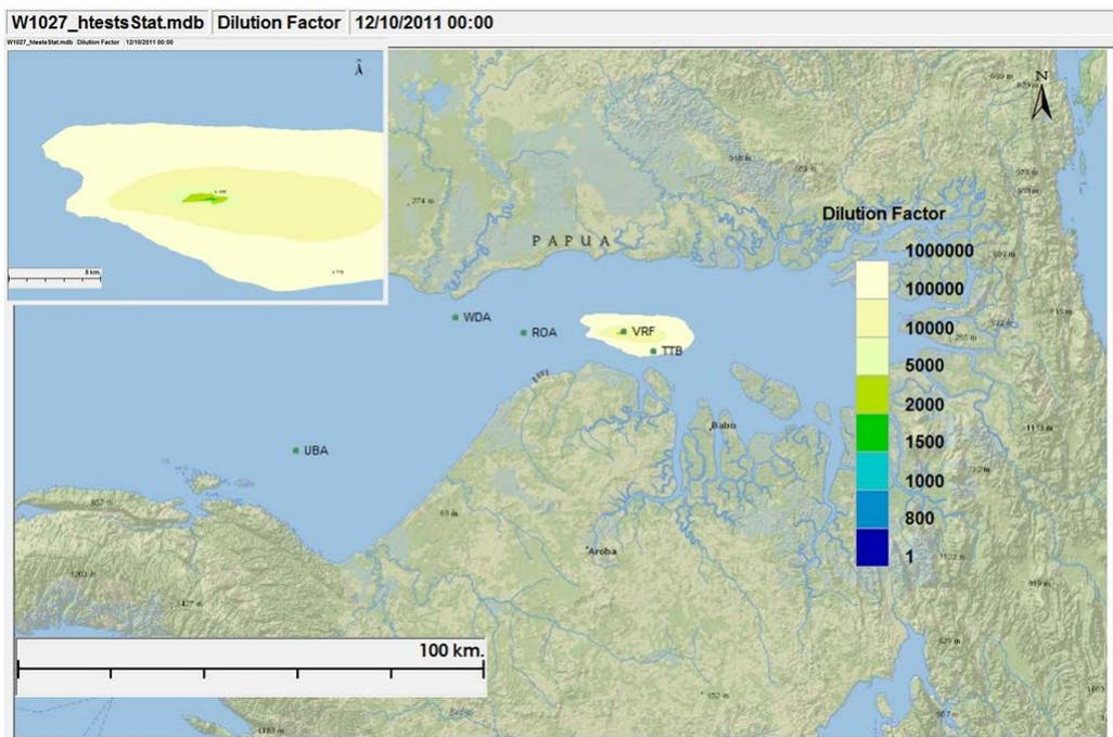
**Figure III-21 Minimum Dilution Factor Contour Plot of Hydrotest Water Discharge at VRF during the Wet season**
