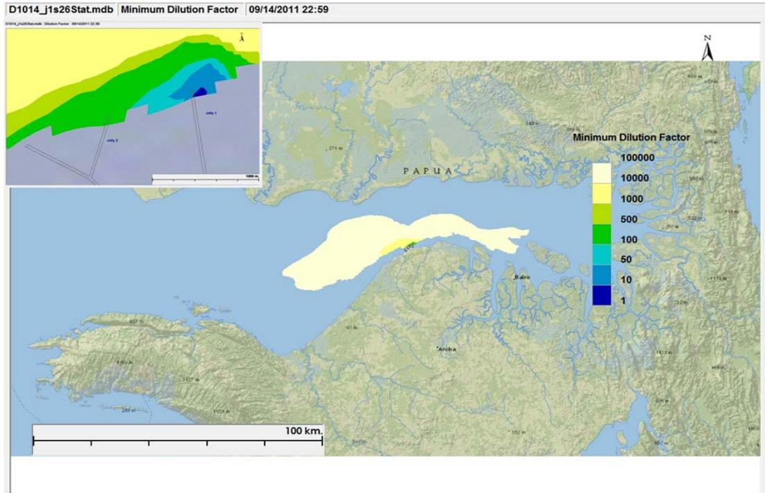
Figure III-52 Contour of Minimum Dilution Factor at LNG 1 Jetty in the Dry Season
