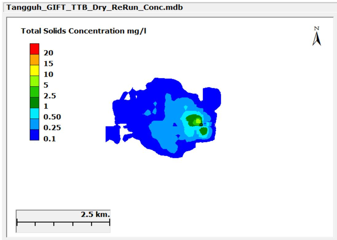
Figure III-5 Maximum Increase in TSS Concentration During Drilling in TTB During the Dry Season
