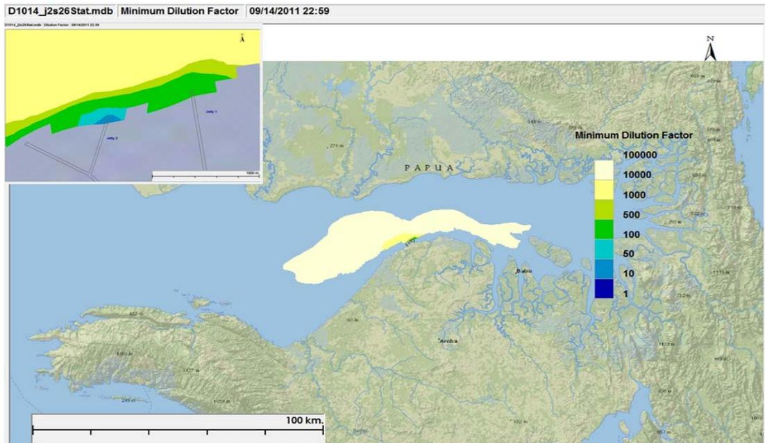
**Figure III-54** Contour of Minimum Dilution Factor at LNG 2 Jetty in the Dry Season
