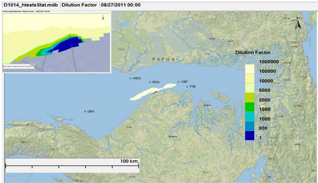
**Figure III-24** Minimum Dilution Factor Contour Plot of the Combined Hydrotest Water and Comingled Wastewater Discharge at the LNG Jetty 1 during the Dry Season
