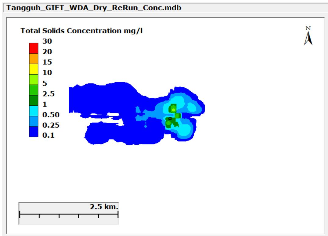
**Figure III-7** Maximum Increase in TSS Concentration During Drilling in WDA During the Dry Season
