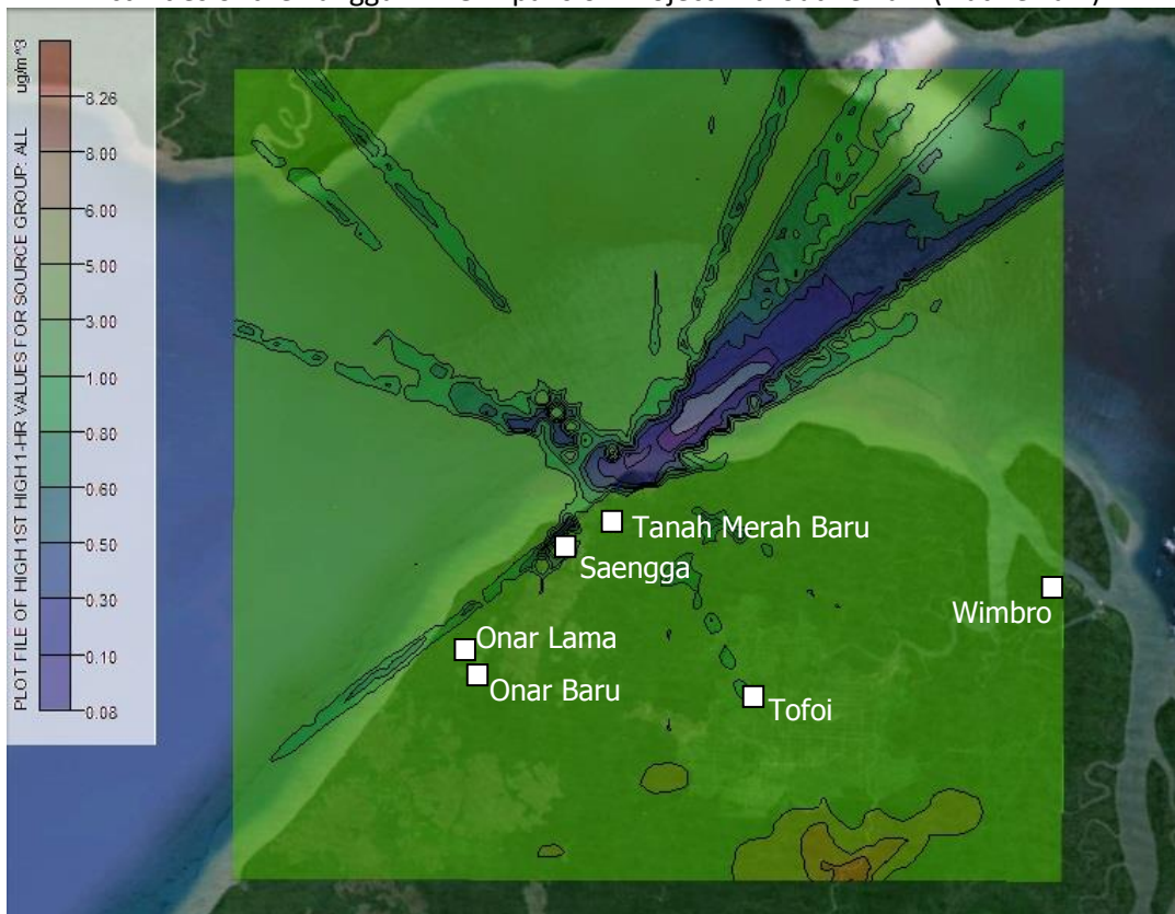
Figure 4.19 Predicted Hourly Average Particulate Concentration Distribution ( \mu\text{g}/\text{m}^3 ) from the Operational Activities of the Tangguh LNG Expansion Project with Terrain (Elevated Terrain)
