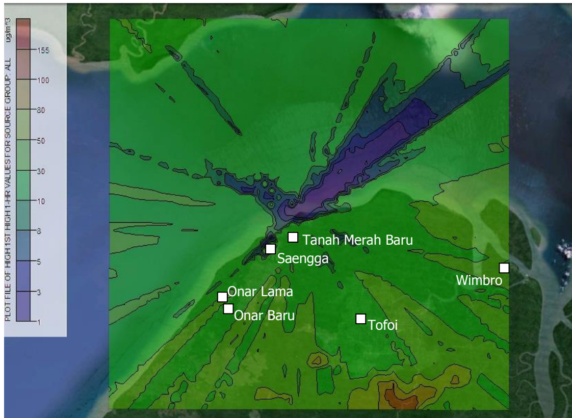
Figure 4.1 Predicted Hourly Average NO 2 Concentration Distribution (µg/m 3 ) from the Operational Activities of the Tangguh LNG Expansion Project with Terrain (Elevated Terrain)
