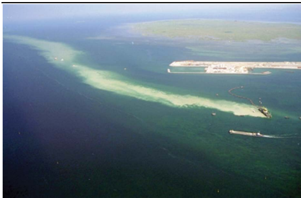
Figure 11.13 Example of a Turbidity Plume Generated by a Cutter Suction Dredger Dredging Coral Structures
