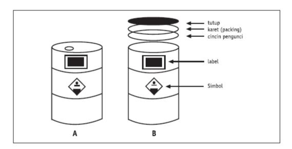
Illustration of waste packaging using drum for: (A) liquid hazardous waste; and (B) sludge or solid hazardous waste
