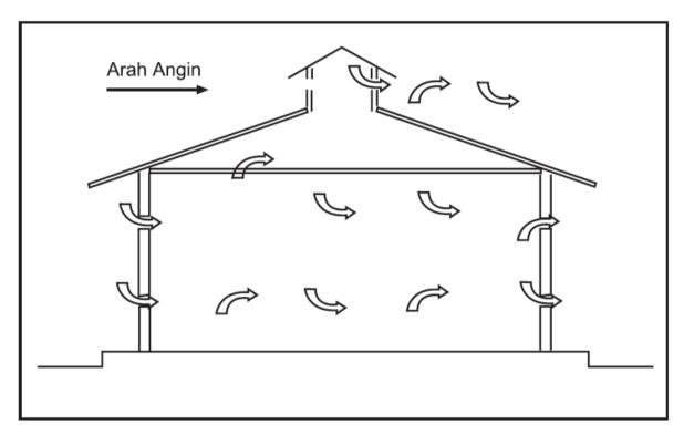
Picture 1: Ventilation System Inside the HAZARDOUS Waste Temporary Storage Building
