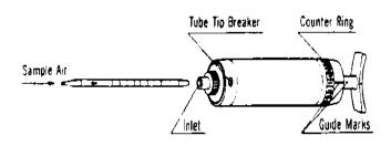
Figure 7.2 Typical Colorimetric Tube Gas Detector
