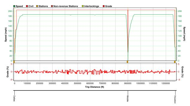
Figure 24: Speed Distance Trip Graph Dallas to Houston Alignment F (186 MPH)
