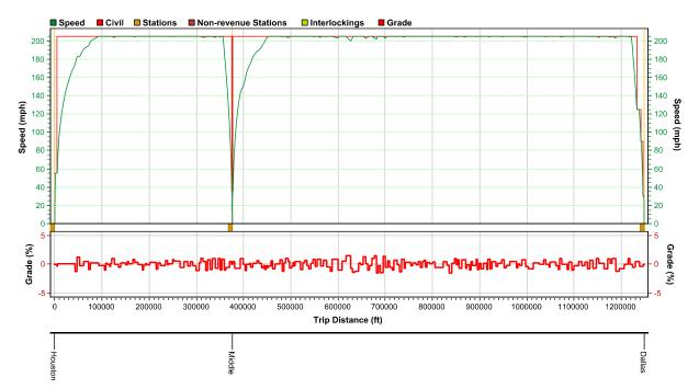
Figure 2: Speed Distance Trip Graph Houston to Dallas Alignment B (205 MPH)
