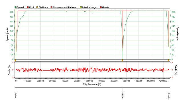
Figure 7: Speed Distance Trip Graph Dallas to Houston Alignment A (205 MPH)
