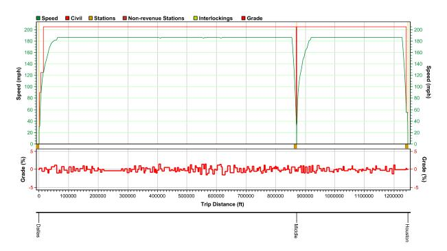
Figure 19: Speed Distance Trip Graph Dallas to Houston Alignment A (186 MPH)
