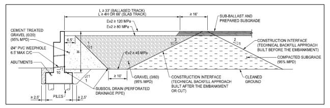
Figure 7: Transition Structure Crossing
