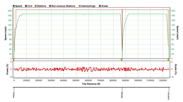
Figure 20: Speed Distance Trip Graph Dallas to Houston Alignment B (186 MPH)
