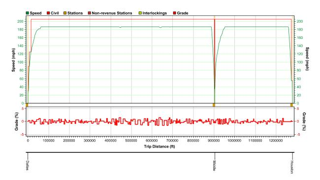
Figure 21: Speed Distance Trip Graph Dallas to Houston Alignment C (186 MPH)
