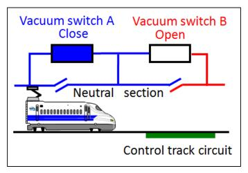
Figure 24: Change-over Switch System Diagram
