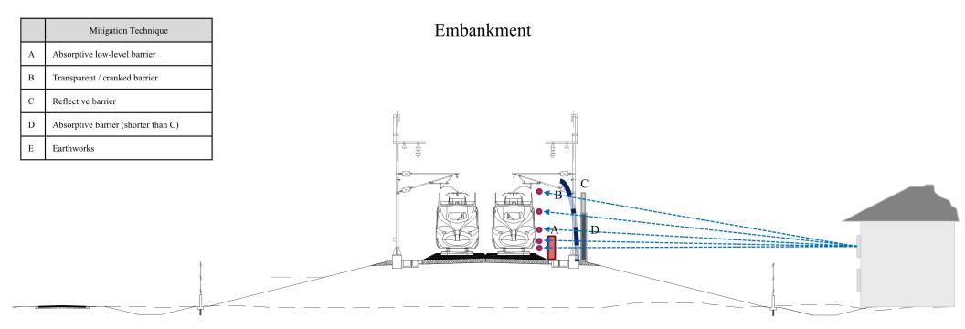
Effectiveness of barriers is height-dependent – must break line-ofsight between source and receiver (i.e. the higher the receiver elevation above the subsource, the taller the barrier will need to be)
