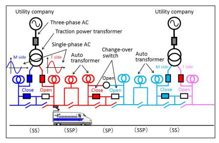
Figure 28: Typical TPSS, SP, SSP Layout
