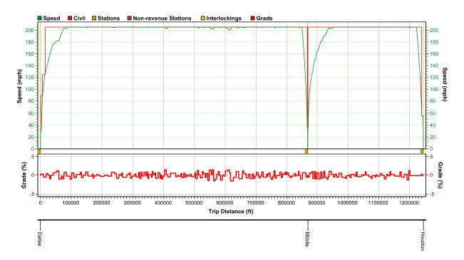
Figure 11: Speed Distance Trip Graph Dallas to Houston Alignment E (205 MPH)
