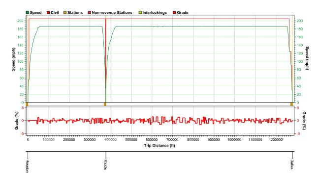
Figure 15: Speed Distance Trip Graph Houston to Dallas Alignment C (186 MPH)
