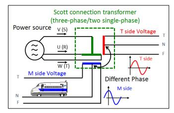
Figure 16: Scott Connection Transformer Diagram
