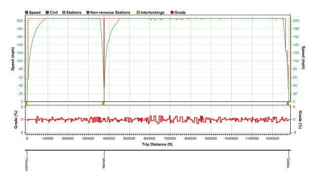
Figure 3: Speed Distance Trip Graph Houston to Dallas Alignment C (205 MPH)
