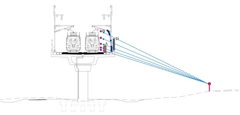
Effectiveness of barriers is height-dependent – must break line-of-sight between source and receiver. In general, viaducts allow for shorter noise barriers.
