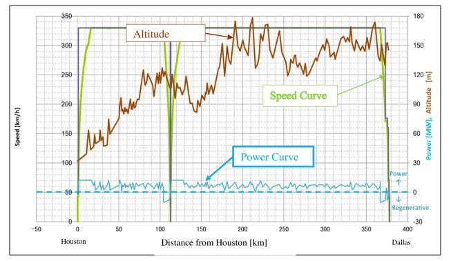
Figure 41: Graph of Speed and Power Consumption vs Distance
