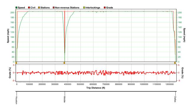
Figure 5: Speed Distance Trip Graph Houston to Dallas Alignment E (205 MPH)
