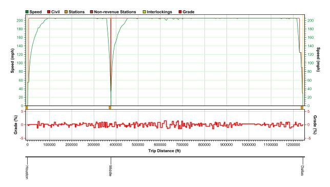
Figure 4: Speed Distance Trip Graph Houston to Dallas Alignment D (205 MPH)
