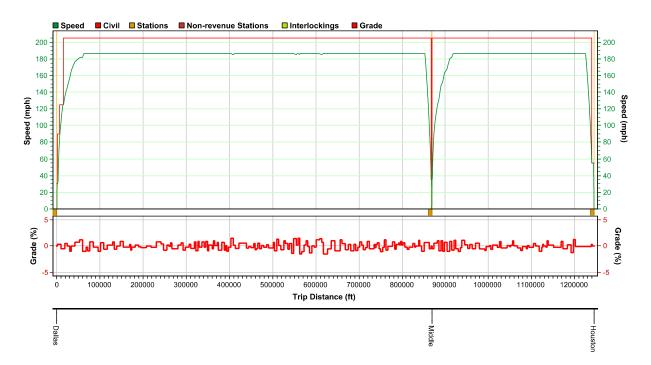
Figure 23: Speed Distance Trip Graph Dallas to Houston Alignment E (186 MPH)
