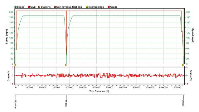
Figure 14: Speed Distance Trip Graph Houston to Dallas Alignment B (186 MPH)
