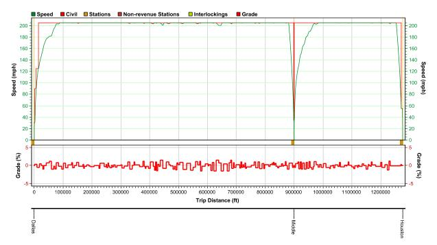
Figure 12: Speed Distance Trip Graph Dallas to Houston Alignment F (205 MPH)
