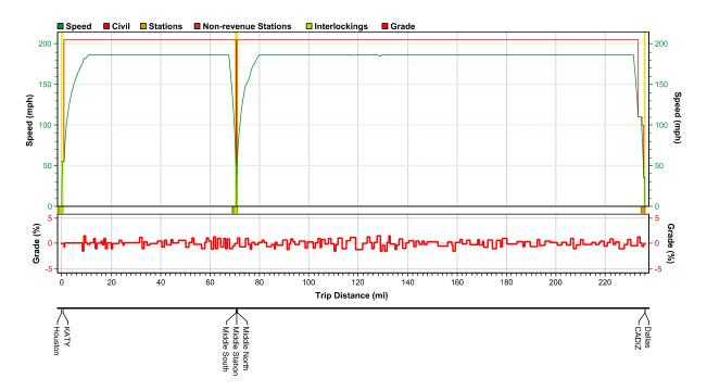
Figure 5: Speed Distance Trip Graph Houston to Dallas Alignment A (186 mph)
