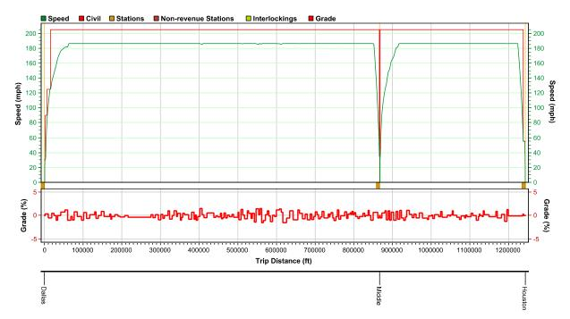
Figure 22: Speed Distance Trip Graph Dallas to Houston Alignment D (186 MPH)
