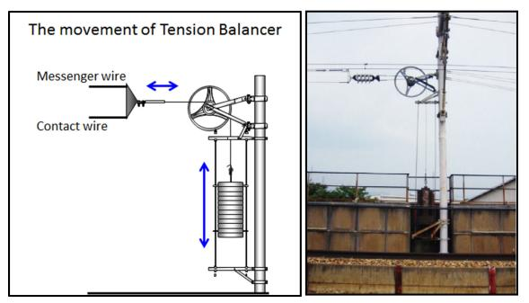
Figure 23: Tension Balancer installed on OCS Pole
