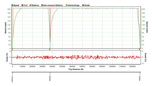
Figure 6: Speed Distance Trip Graph Houston to Dallas Alignment F (205 MPH)
