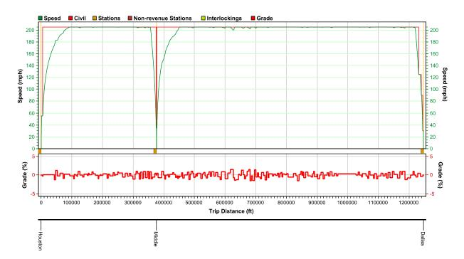
Figure 1: Speed Distance Trip Graph Houston to Dallas Alignment A (205 MPH)
