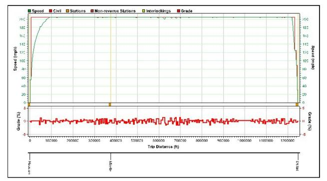
Figure 4: Speed Distance Trip Graph Houston to Dallas Alignment A (205 mph)
