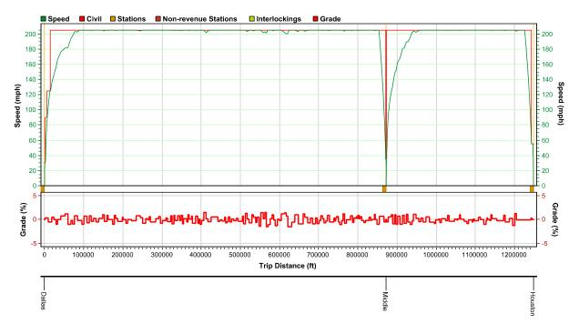
Figure 8: Speed Distance Trip Graph Dallas to Houston Alignment B (205 MPH)
