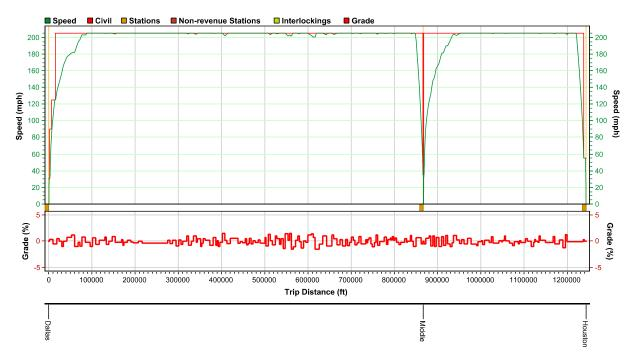
Figure 10: Speed Distance Trip Graph Dallas to Houston Alignment D (205 MPH)
