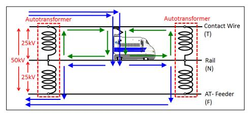
Figure 26: Current Flow Diagram (Autotransformers)
