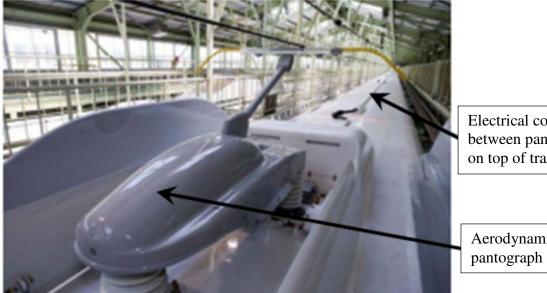
Electrical connection between pantographs on top of train
