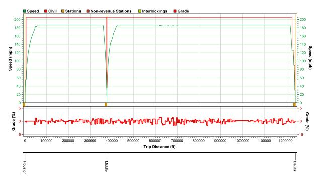
Figure 16: Speed Distance Trip Graph Houston to Dallas Alignment D (186 MPH)
