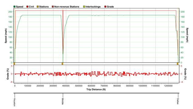
Figure 18: Speed Distance Trip Graph Houston to Dallas Alignment F (186 MPH)
