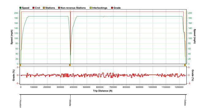
Figure 13: Speed Distance Trip Graph Houston to Dallas Alignment A (186 MPH)
