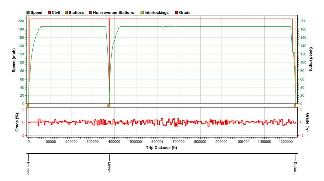
Figure 17: Speed Distance Trip Graph Houston to Dallas Alignment E (186 MPH)
