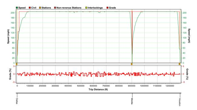
Figure 9: Speed Distance Trip Graph Dallas to Houston Alignment C (205 MPH)
