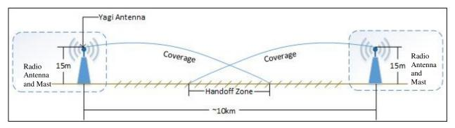
Figure 29: Typical Mast Spacing with Antenna Mounting Height of 50ft (15m) above TOR
