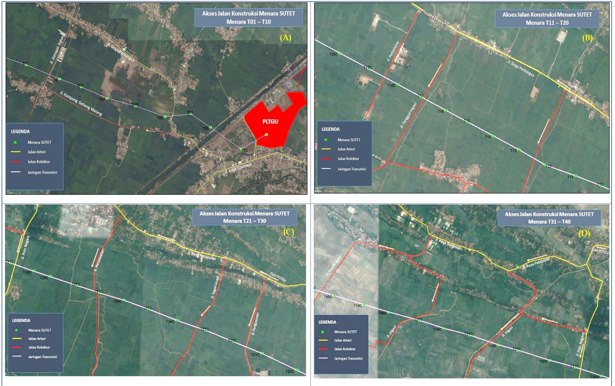
Gambar 3-13 Akses Jalan Konstruksi PLTGU, Jaringan Transmisi (A) Tower T01-T10; (B) Tower T11-T20; (C) Tower T21-T30; (D) Tower T31-T40
