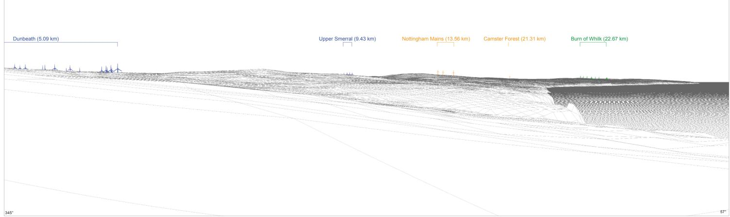
Computer generated wireframe showing consented wind farm turbines in green, application wind farm turbines in blue and scoping wind farm turbines in orange
