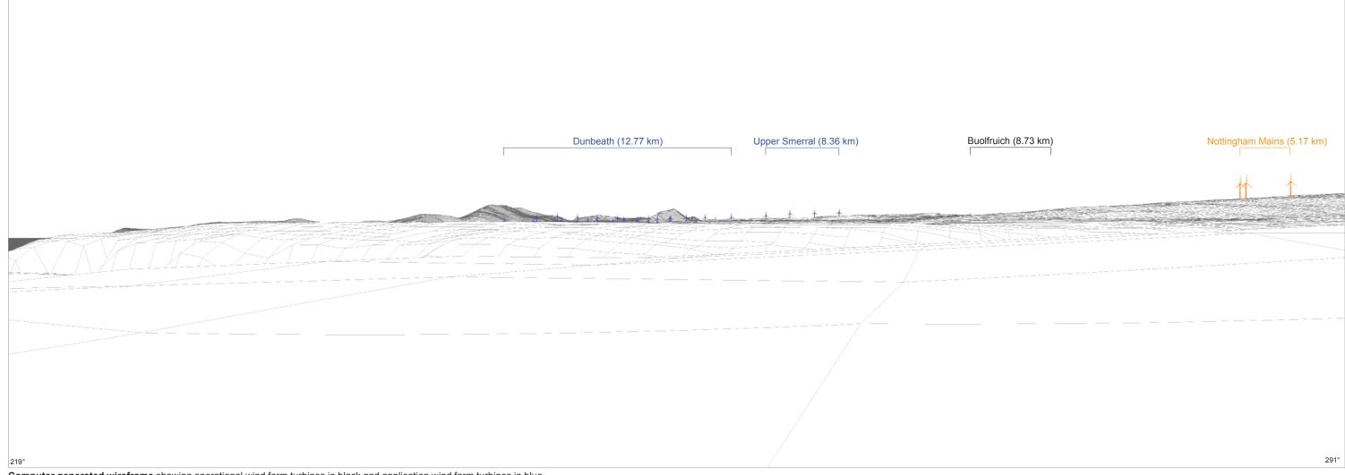
Computer generated wireframe showing operational wind farm turbines in black and application wind farm turbines in blue
