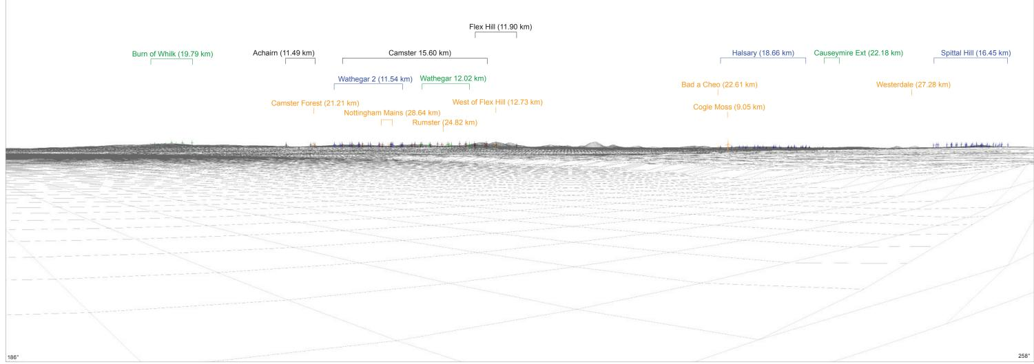
Computer generated wireframe showing operational wind farm turbines in black, consented wind farm turbines in green, application wind farm turbines in blue and scoping wind farm turbines in orange
