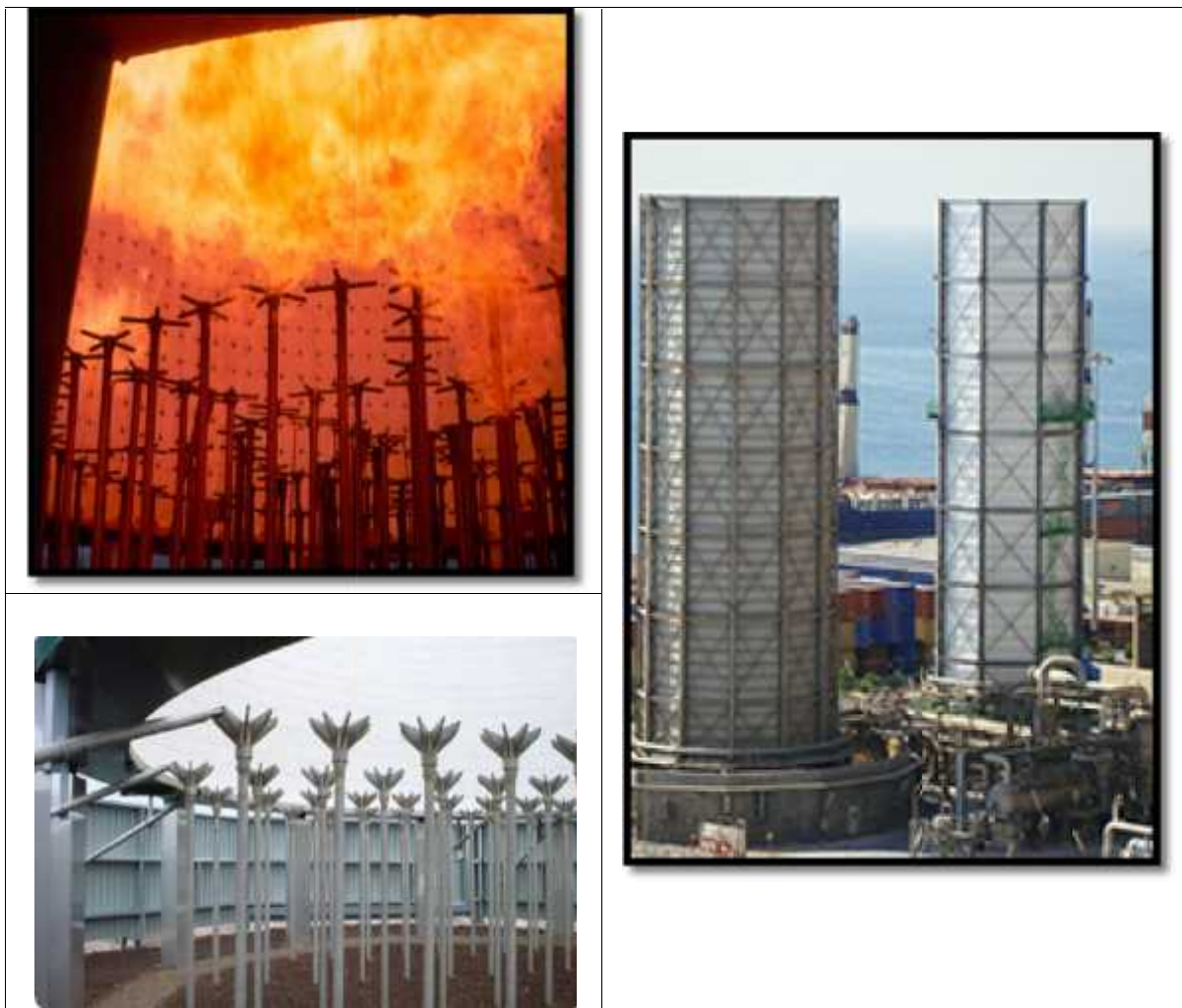
Gambar 1.46. Enclosed Ground Flare with Chamber Cast Burner Heads
