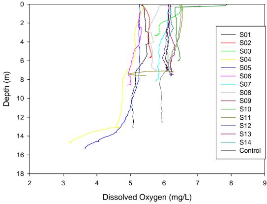
Figure 32: Seawater dissolved oxygen profiles
