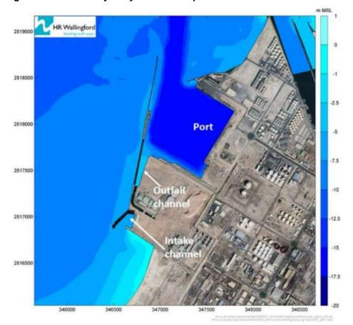
Figure 48: Model bathymetry close to the plant
