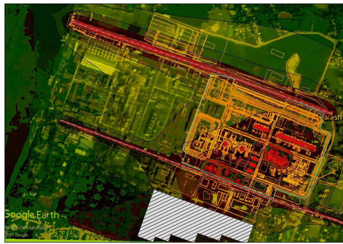
Figure 7.10: Noise Propagation Modeling during Daytime
