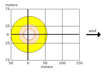
Figure 10.2: Thermal rediation from jet fire
