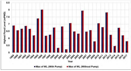
Figure 7.5: Highest Flood Level With and Without Pump
