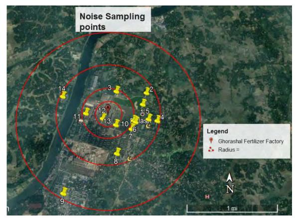
Figure 6.24: Sampling points of noise levels around the project site
