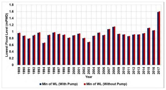
Figure 7.6: Lowest Flood Level With and Without Pump
